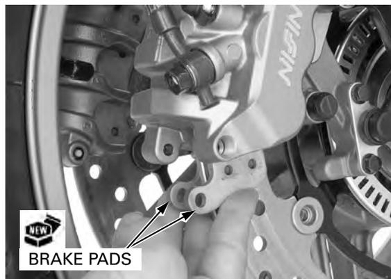
Coat the stopper ring on the pad pin end with the silicone grease
