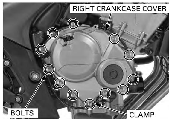
*The lifter lever spindle is engaged with the clutch lifter piece inside of the right crankcase cover.*
