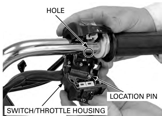
Tighten the forward screw first, then the rear screw.
