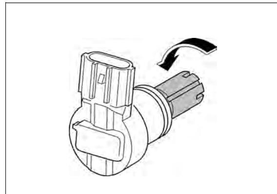
Apply oil to new O-ring and install it to the IACV motor.
