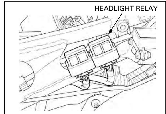
Connect the ohmmeter to the headlight relay connector terminals.
