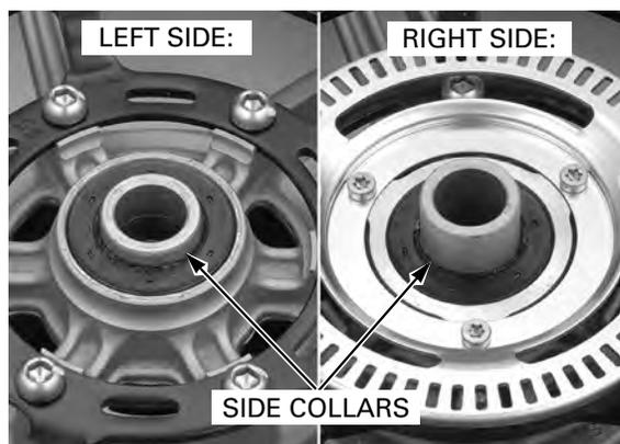
Apply thin layer of grease to the front axle surface.
