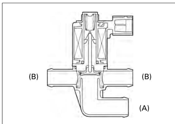
Check the resistance between the terminals of the PAIR control solenoid valve.
