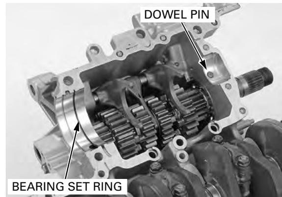
Install the countershaft by aligning the countershaft bearing groove with the set ring on the crankcase, and bearing cap hole with the dowel pin.
