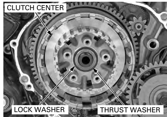
Remove the thrust washer.
