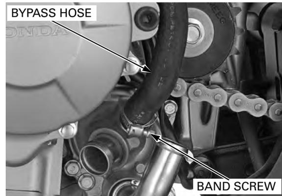
Connect the lower, upper radiator hose. Tighten the hose band screws as shown.
