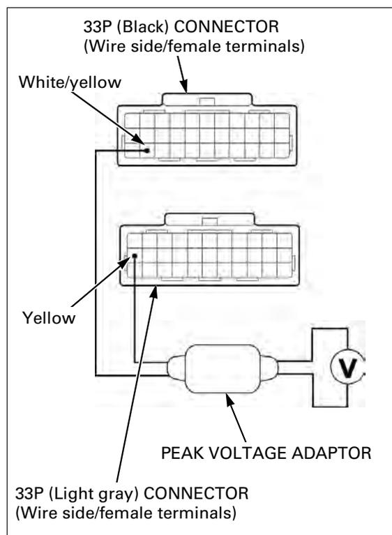
Disconnect the CKP sensor 2P (Red) connector and connect the tester probes to the terminal (Yellow and White/yellow).
