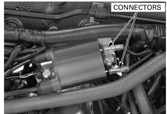
Disconnect the PAIR control solenoid valve 2P (Black) connector.
