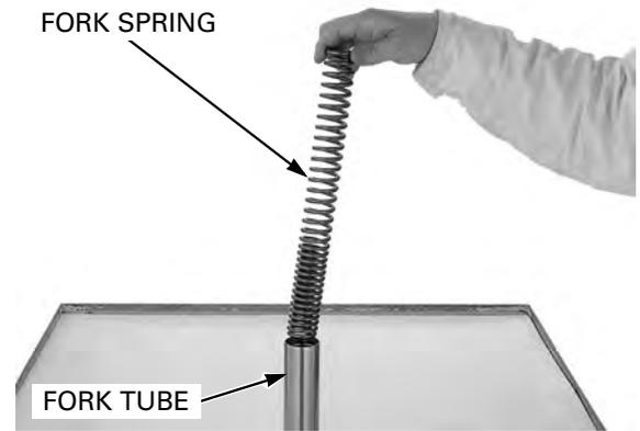
Pour out the fork fluid by pumping the fork tube several times.
