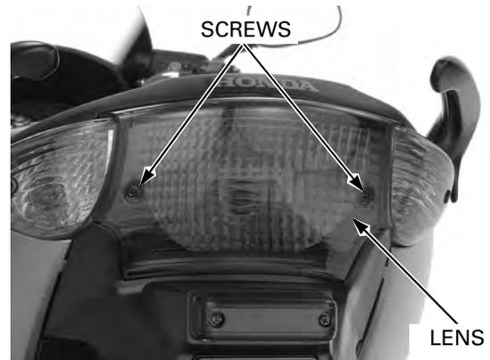
While pushing in, the tail/brake light bulb counter-clockwise to remove it and replace with a new one.
