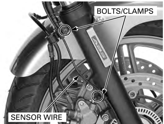
Remove the wheel speed sensor mounting bolts.
