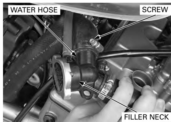
Install the filler neck and tighten the bolt securely. Connect the #4 spark plug cap securely.
