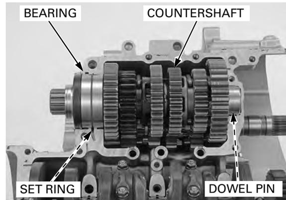
Also align the countershaft bearing stopper pin with the groove in the crankcase.
