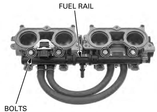
Connect the MAP sensor vacuum hoses and IDC solenoid valve air hoses.
