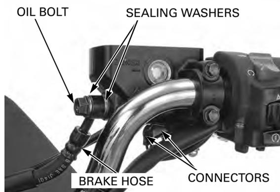
Remove the bolts from the master cylinder holder and remove the master cylinder assembly.
