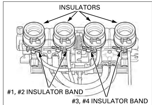
Tighten the throttle body side insulator band screws so that the width between the band ends is  $7 \pm 1$  mm ( $0.28 \pm 0.04$  in).
