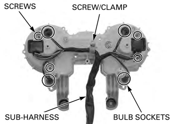
Remove the speedometer, tachometer and indicator plate.
