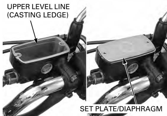
Fill the rear brake reservoir to the upper level line with DOT 4 brake fluid.
