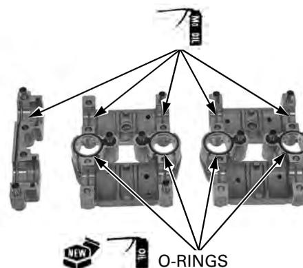
Note the correct locations with the identification marks as shown.
