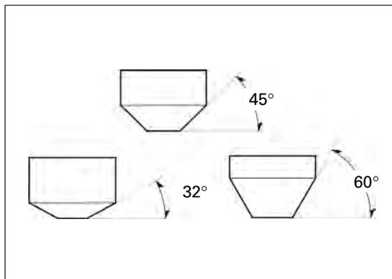
If the contact area is too high on the valve, the seat must be lowered using a 32-degree flat cutter.
