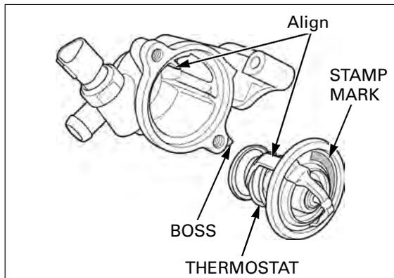
Install the thermostat housing cover to the housing by aligning the bosses of housing and cover. Tighten the bolts to the specified torque.
