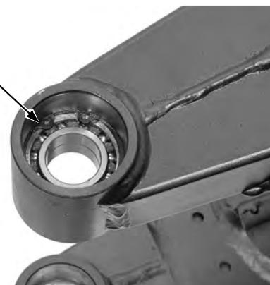
Press the right pivot radial ball bearings out using the special tool and a hydraulic press.
