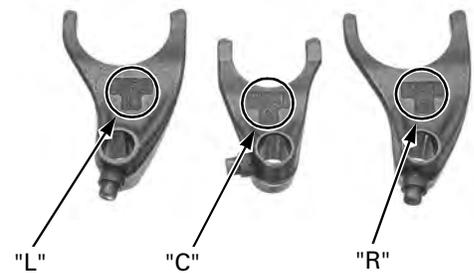
Install the shift forks into the shift drum guide grooves with the identification marks facing toward the right side of the engine and insert the fork shaft.
