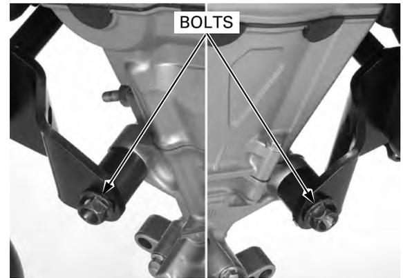
Mount the radiator with the mounting bolt and washer to the front engine hanger.
