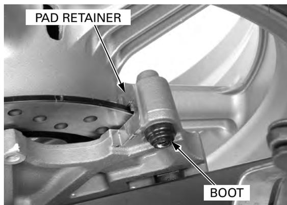
Remove the pad spring, collar and caliper sub slide pin boot from the caliper body.
