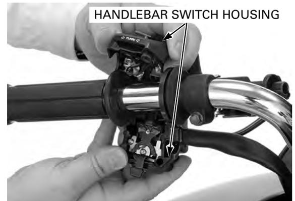
Remove the left handle grip and switch housing plate.
