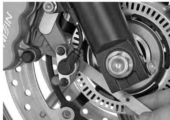
**2. Speed Sensor Condition Inspection**
