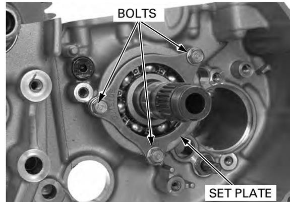
Remove the mainshaft bearing from the crankcase.
