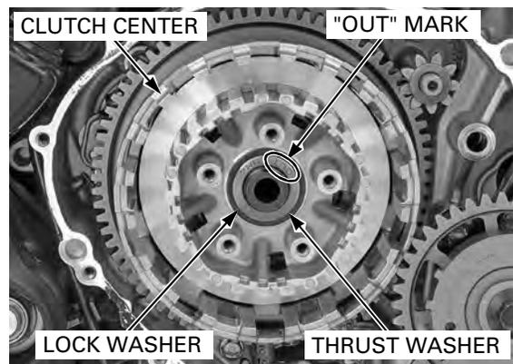
Apply engine oil to the threads and seating surface of a new clutch center lock nut, then install it onto the mainshaft.
