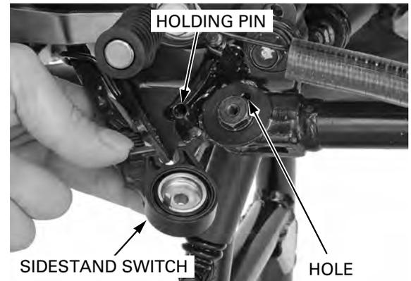
Secure the sidestand switch with a new bolt.
