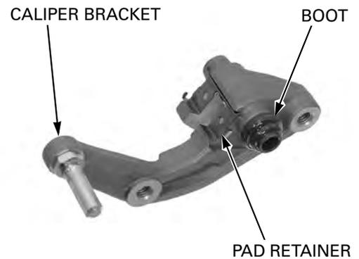
Apply silicone grease to the caliper and bracket pins and install the caliper bracket over the caliper body.
