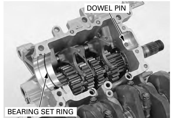
Remove the shift drum bearing set bolts/washers.
