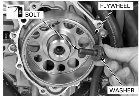
Hold the flywheel using the special tool, then tighten the bolt to the specified torque.
