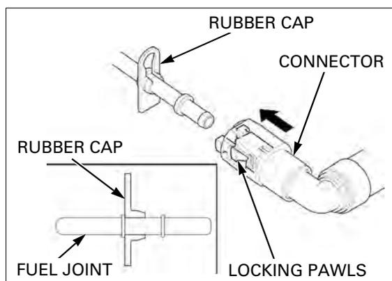
3. Make sure the connection is secure and that the pawls are firmly locked into place; check visually and by pulling the connector.
