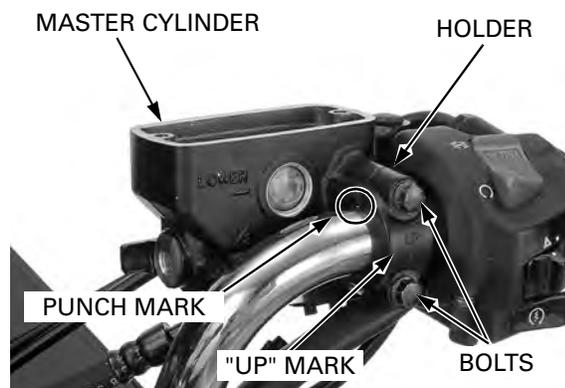
Connect the brake hose to the master cylinder with the oil bolt and new sealing washers.
