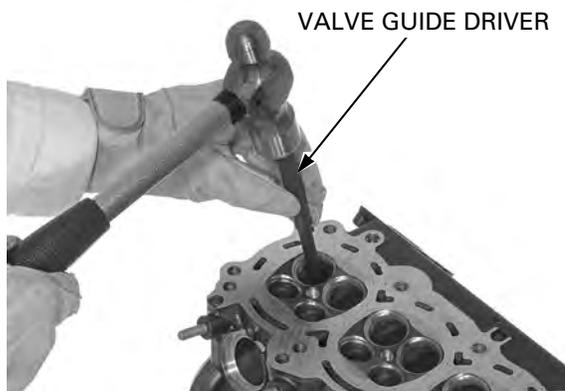
Drive in the guides to the specified depth from the top of the cylinder head.
