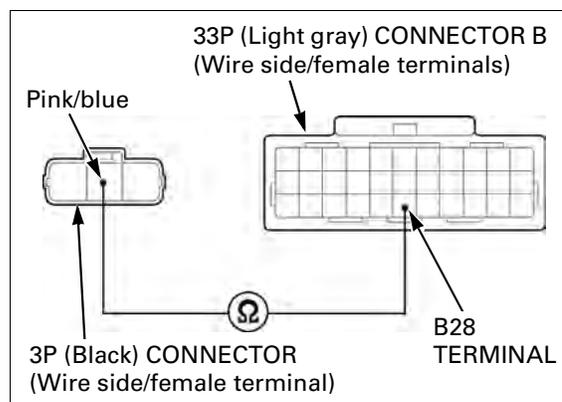
**5. VS Sensor Pulse Line Short Circuit Inspection**
