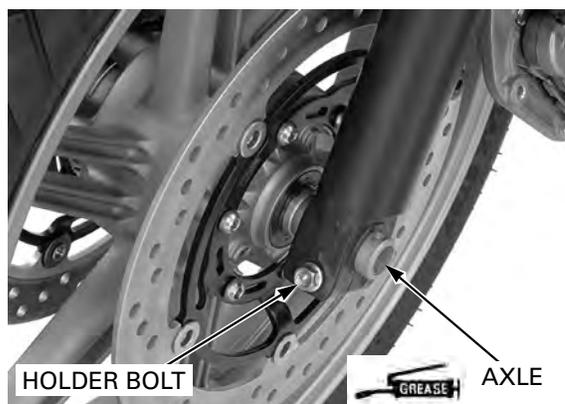
Hold the axle and tighten the axle bolt to the specified torque.
