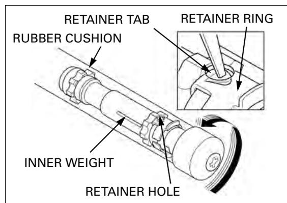
Remove the grip end from the handlebar weight.
