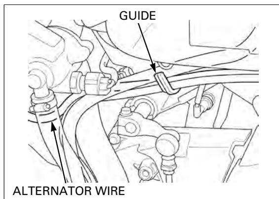
*The alternator cover (stator) is magnetically attached to the flywheel, be careful during removal.*
