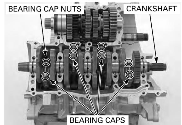
Remove the main journal bearings from both the crankcase halves.
