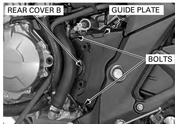
Set the sidestand switch wire clip to the hole of rear cover B.
