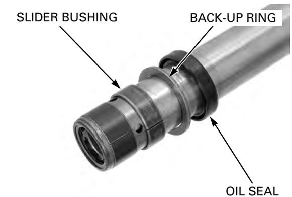
*Do not remove the fork tube bushing unless it necessary to replace it with a new one.*
