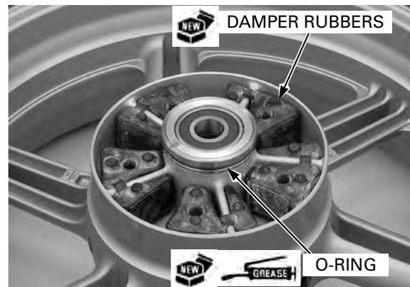
Apply grease to the driven flange and rear wheel hub contact area.
