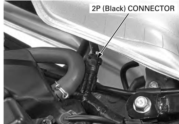
Turn the ignition switch ON and measure the voltage between the terminals.
