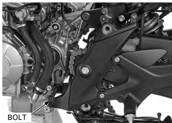
Install the collar between the engine and rear engine hanger.
