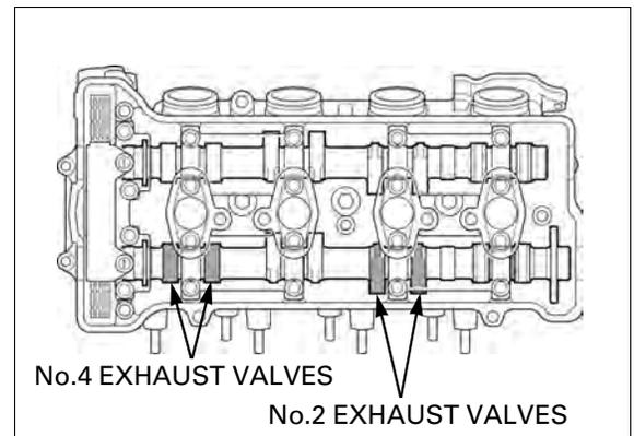
Turn the crankshaft clockwise 1/2 turn (180°), align the "T" mark on the CKP sensor rotor with the index mark on the right crankcase cover.
