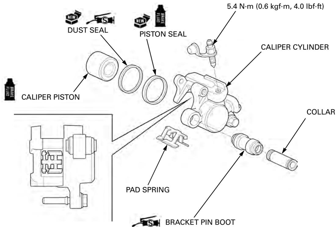
Coat the new piston seal with clean brake fluid.
