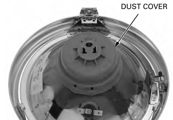
*Avoid touching halogen headlight bulb. Finger prints can create hot spots that cause a bulb to break.*
