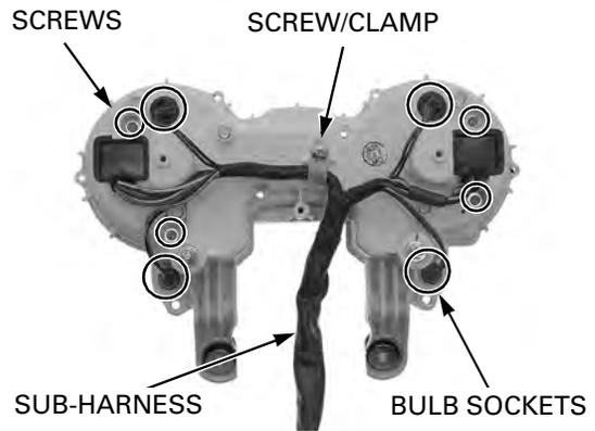
Install the front cover to the combination meter case, then tighten the screws securely.
