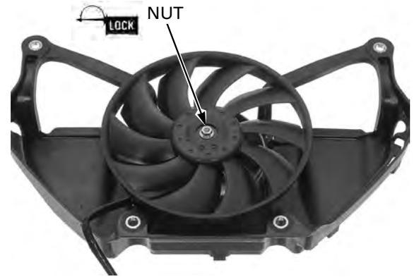
Install the cooling fan motor assembly onto the radiator.
