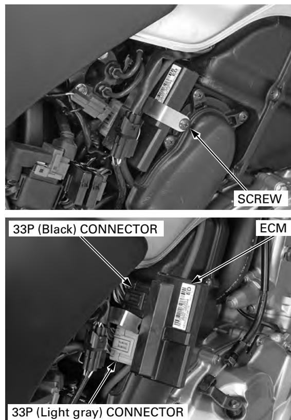
**ECM POWER/GROUND LINE INSPECTION****ENGINE DOES NOT START (No DTC and MIL blinking)****1. ECM Power Input Voltage Inspection**
