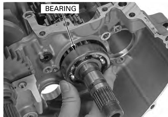
Apply a locking agent to the set plate bolt threads. Install the mainshaft bearing set plate with its "OUT SIDE" mark facing out.
