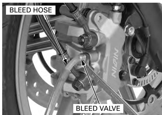
Connect a bleed hose to the rear caliper bleed valve.
