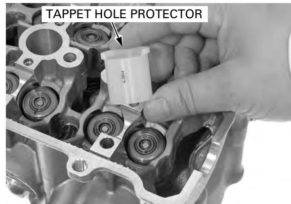
An equivalent tool can easily be made from a plastic 35 mm film container as shown.
