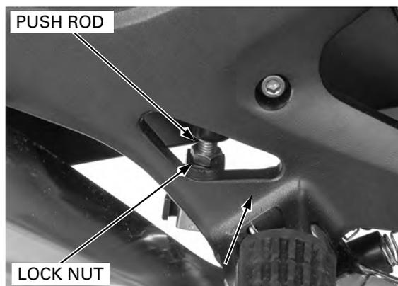
If the brake pedal is adjusted to the lower position, make sure that the clearance between the lower end of the push rod and the brake pedal does not fall below 1 mm (0.04 in).
