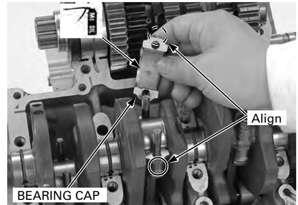
Apply engine oil to the connecting rod bearing cap nut threads and seating surfaces, and install them.
