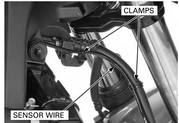
Remove the bolts and release the sensor wire from the clamps.
