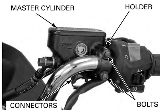
Remove the right handlebar switch/throttle housing screws.
