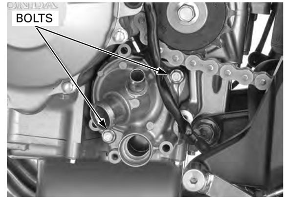
Install the water pump cover assembly bolts. Tighten the assembly bolts to the specified torque.
