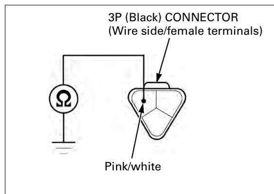
**FUEL SYSTEM (PGM-FI)****MIL 8 BLINKS (TP SENSOR)**
