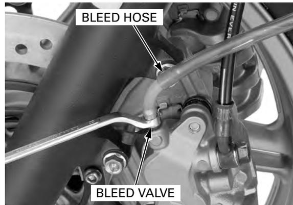
Fill the reservoir with DOT 4 brake fluid from a sealed container.
