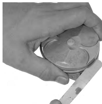
*Push the rings into the cylinder with the top of the piston to be sure they are squarely in the cylinder.*
