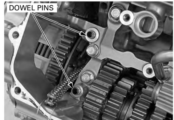
Remove the bolts, oil pipe B and O-rings.
