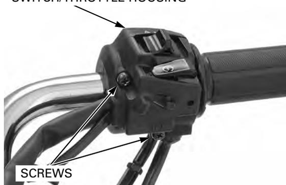
Disconnect the throttle cable ends from the throttle pipe and remove the right handlebar switch/throttle housing.
