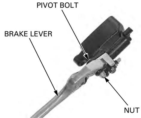
Remove the screw and brake light switch.
