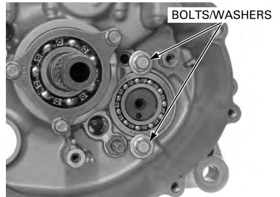
Remove the fork shaft and shift forks.
