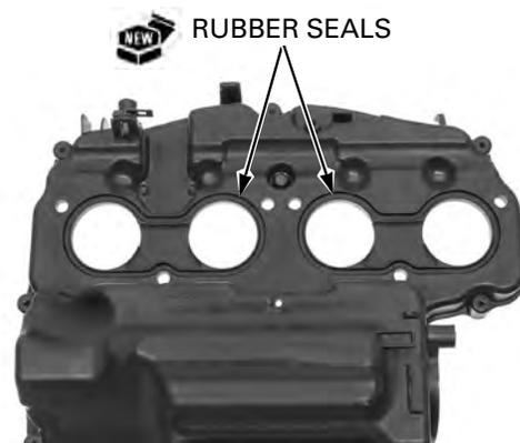
Install the lower air cleaner housing onto the throttle body, then install the air funnels.
