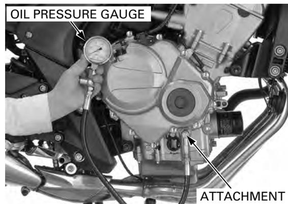
Check the oil level and add the recommended oil if necessary (page 3-15).
