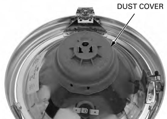
Connect the headlight bulb sockets to the head light bulbs.
