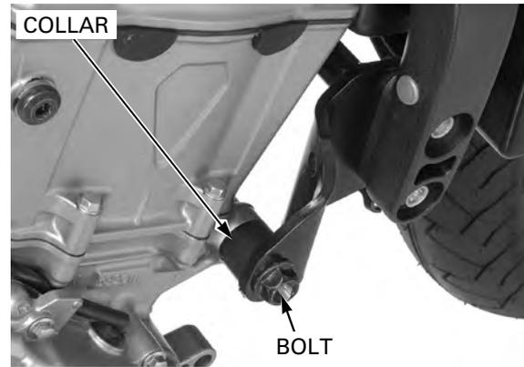
Install the left front engine mounting bolt and collar.
