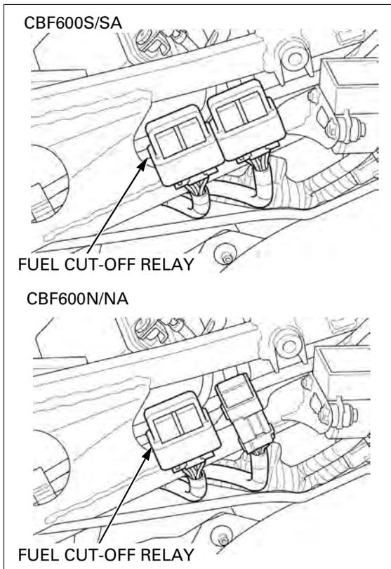
Jump the Brown and Black/white wire terminals of the wire harness side using a jumper wire.
