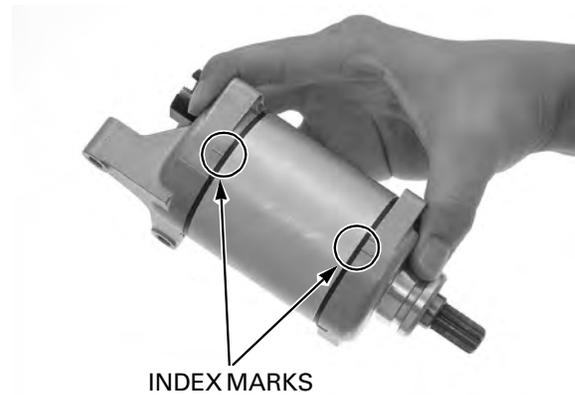
Tighten the case bolts securely.
