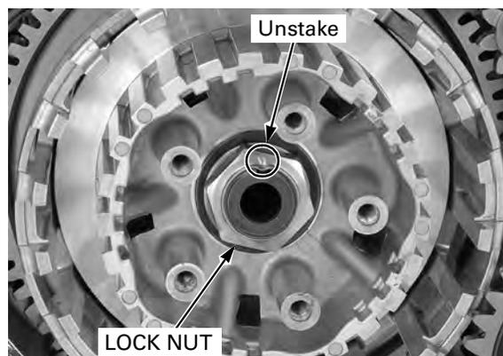
Hold the clutch center with the special tool and remove the clutch center lock nut.
