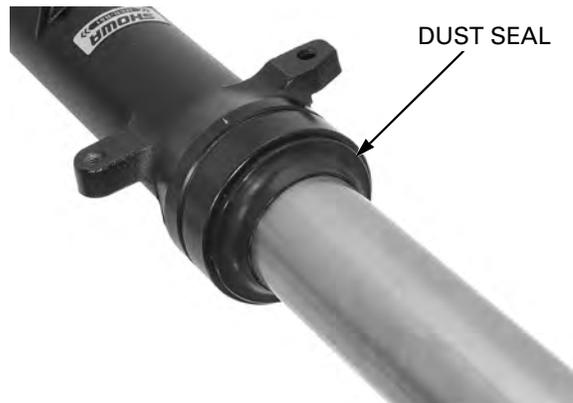
*Do not scratch the fork tube sliding surface.*
