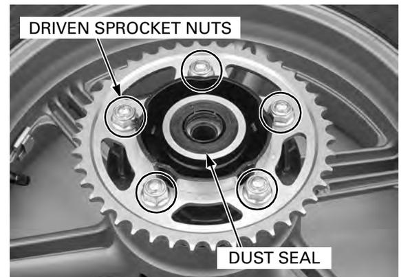
Remove the driven flange assembly from the left wheel hub.
