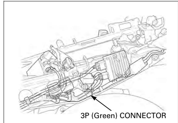
Remove the screws, washers and bank angle sensor.
