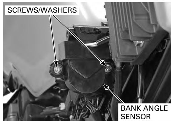
Place the bank angle sensor horizontal as shown, and turn the ignition switch ON and engine stop switch "O".
