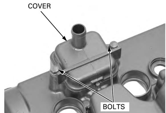
Remove the PAIR check valves from the cylinder head cover.
