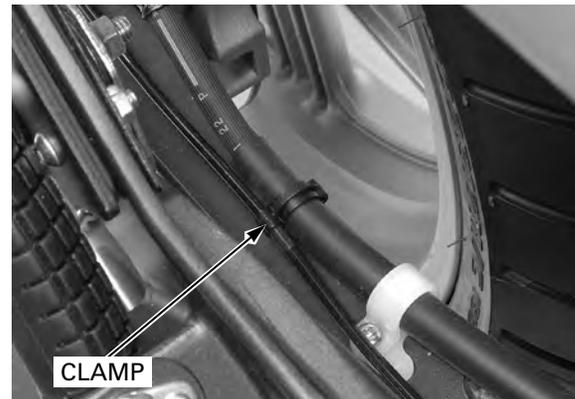
Release the sensor wire clips from the caliper bracket.
