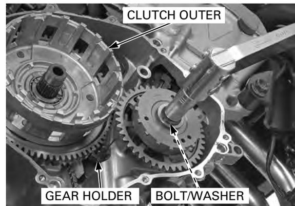
Tighten the starter clutch mounting bolt to the specified torque.
