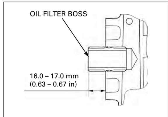
Apply clean engine oil to new oil filter cartridge threads and O-ring.
