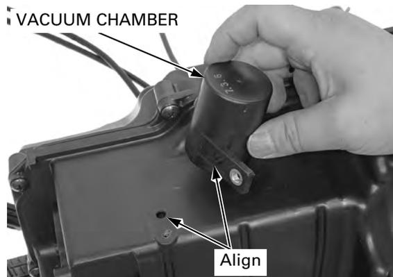
Tighten the vacuum chamber screw securely.
