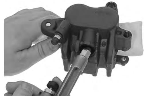
*Be careful not to damage the piston sliding surface.*
