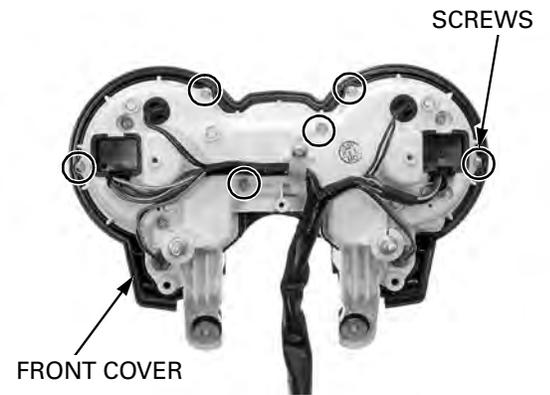
Remove the meter screws.
