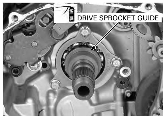
Apply oil to the oil pump drive/driven sprocket teeth and drive chain.
