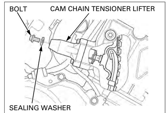
*Failure to release the cam chain tensioner will result in inaccurate valve clearance reading.*
