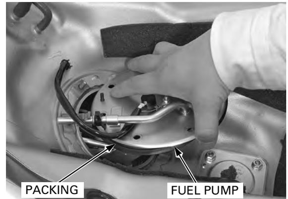
Remove the fuel pump chamber from fuel pump unit.
