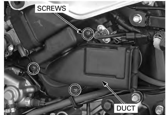
Remove and inspect the air cleaner element in accordance with the maintenance schedule (page 3-4).
