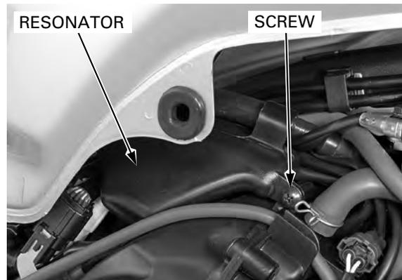
*Refer to the wires properly (page 1-24).* Route the fuel feed hose to the guide of front resonator.
