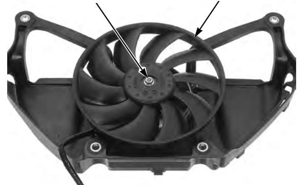
Release the fan motor wire from the guide of fan motor shroud.
