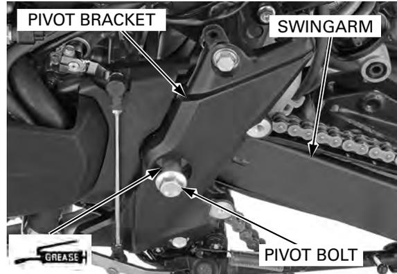
Remove the swingarm pivot nut and washer.
