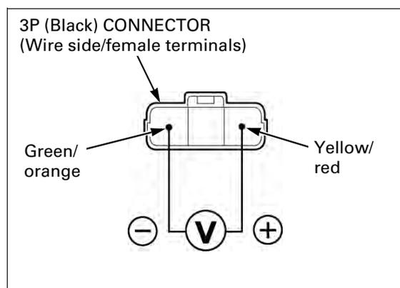
**FUEL SYSTEM (PGM-FI)****3. ECM Output Voltage Inspection**
