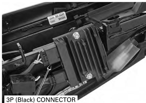
Release the alternator wire from the clamps.
