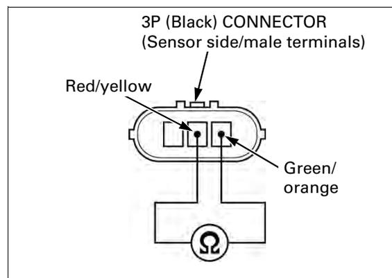
**4. TP Sensor Input Voltage Inspection**
