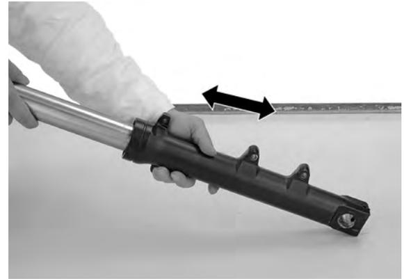
Remove the oil lock piece from the fork slider.
