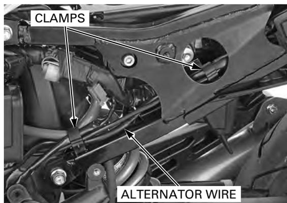
Unhook the alternator wire from the guide.
