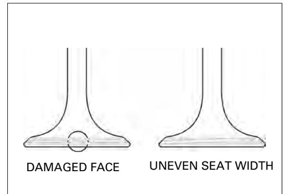
*The valves cannot be ground. If a valve face is burned or badly worn or if it contacts the seat unevenly, replace the valve.*
