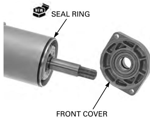
Align the index marks on the front cover, starter motor case and rear cover.
