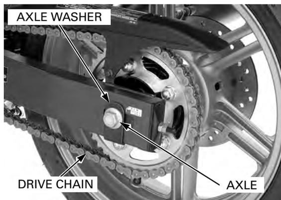
Install the axle washer, nut and axle nut.
