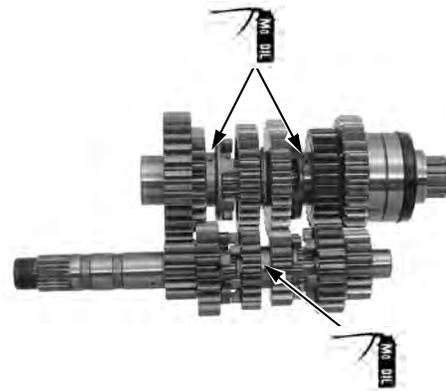
Install the mainshaft into the crankcase.
