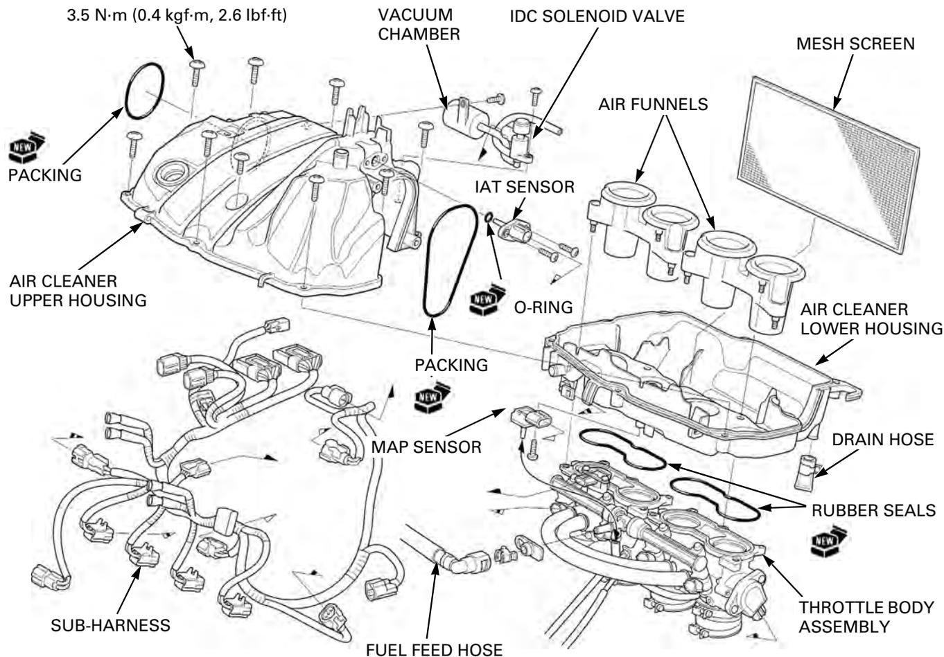
Install new rubber seals into the lower air cleaner housing.
