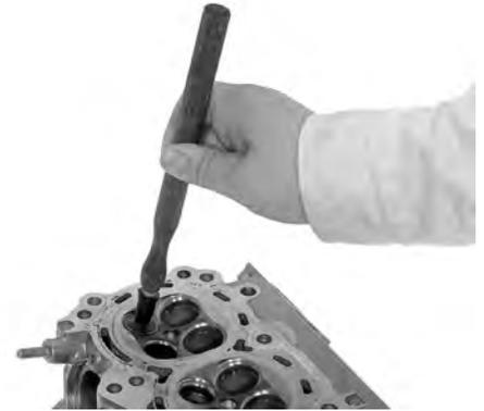
Remove the valve and inspect the valve seat face. The valve seat contact should be within the specified width and even all around the circumference.
