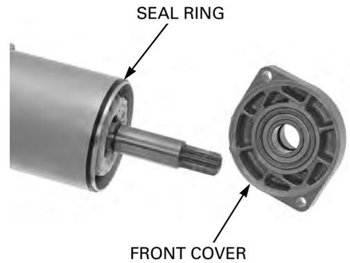
Remove the starter motor case and seal ring.
