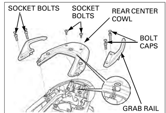
Remove the socket bolts and special bolts/collars.
