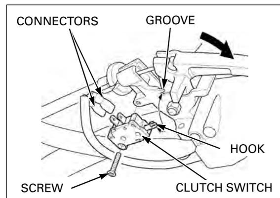
Apply grease to the clutch cable end. Connect the clutch cable end to the clutch lever and tighten the lock nut.
