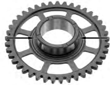
Check the starter reduction gear for wear or damage and replace it if necessary.
