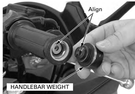
Install and tighten the screw securely.
