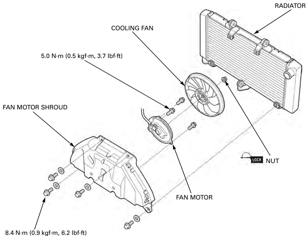
Install the fan motor onto the fan motor shroud and tighten the mounting bolts to the specified torque.
