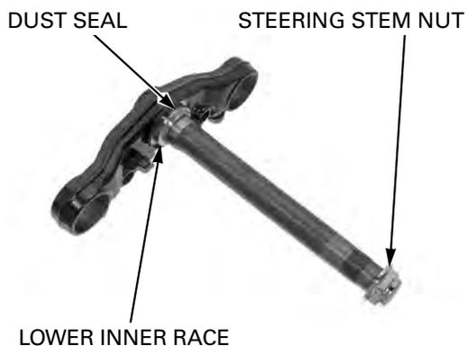
Apply grease to a new dust seal lips and install it over the steering stem. Install a new lower bearing inner race using a special tool and a hydraulic press.
