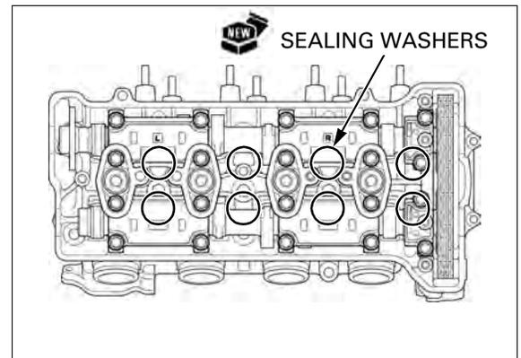
Gradually tighten the camshaft holder bolts until the camshaft holders lightly contact the cylinder head surface.
