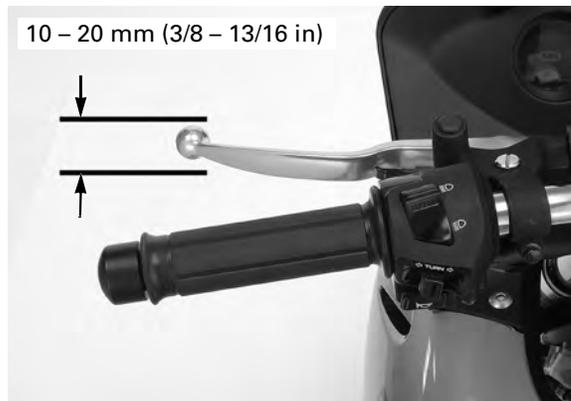
Minor adjustment is made using the upper adjuster at the clutch lever.
