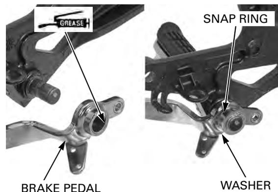
Install the joint pin. Secure the master cylinder with a new cotter pin. Install the switch spring and brake pedal return spring in the direction as shown.
