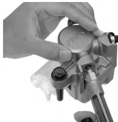
*Be careful not to damage the piston sliding surface.*
