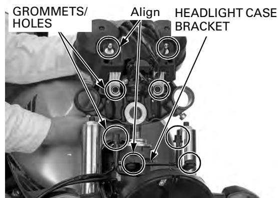
Install and tighten the stem nut to the specified torque.
