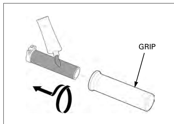
Apply grease to the throttle pipe flange groove and sliding surfaces.
