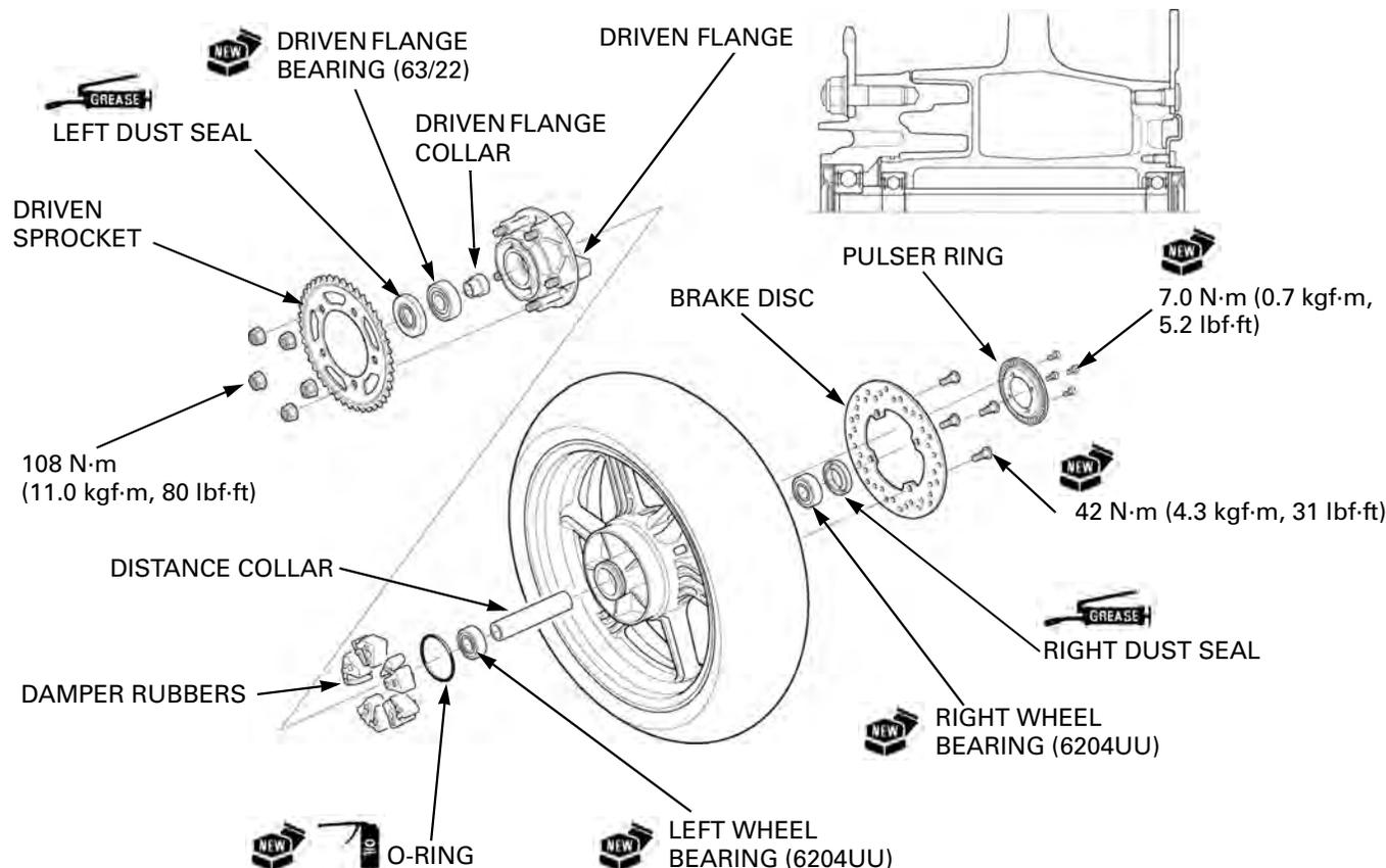
Never install the old bearings, once the bearings has been removed, the bearing must be replaced with new ones.
