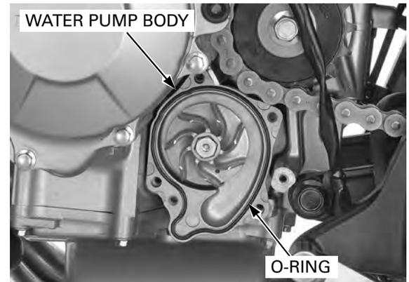
Remove the O-ring from the water pump body.
