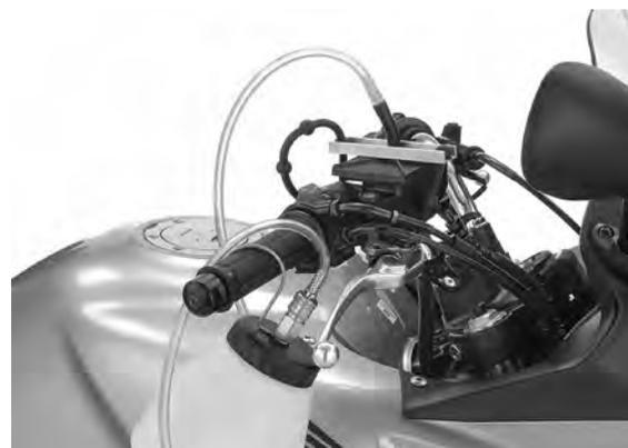
Connect a commercially available brake bleeder to the right caliper upper bleed valve.
