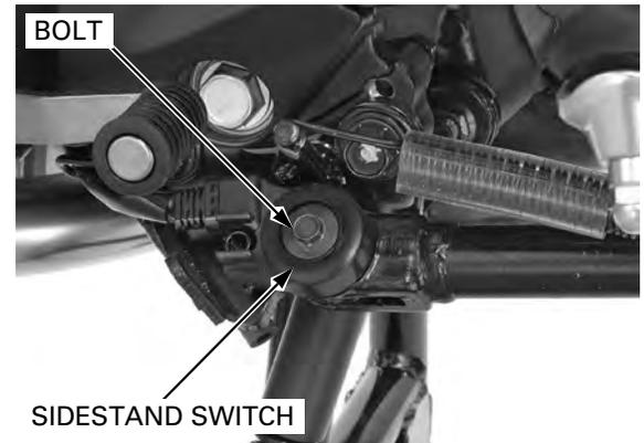
Install the sidestand switch by aligning the switch pin with the sidestand hole and the switch groove with the holding pin.
