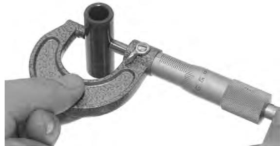
Measure the diameter of the piston at 6 mm (0.2 in) from the bottom and 90 degrees to the piston pin hole.
