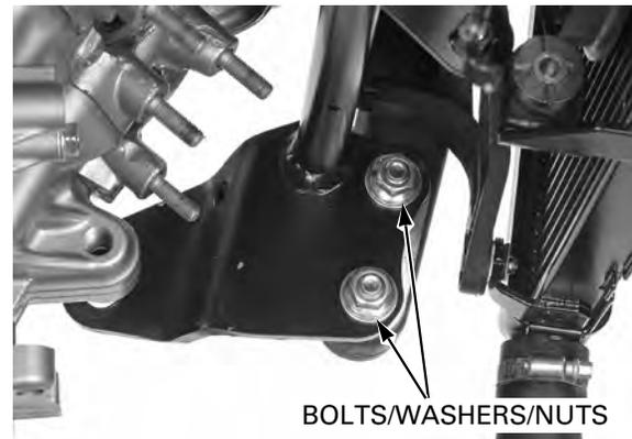
Remove the right front engine hanger bracket bolts, washers, nuts and release the horn wire.
