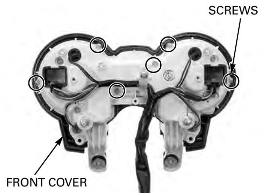
Install the lower cover to the combination meter case, then tighten the screws securely.
