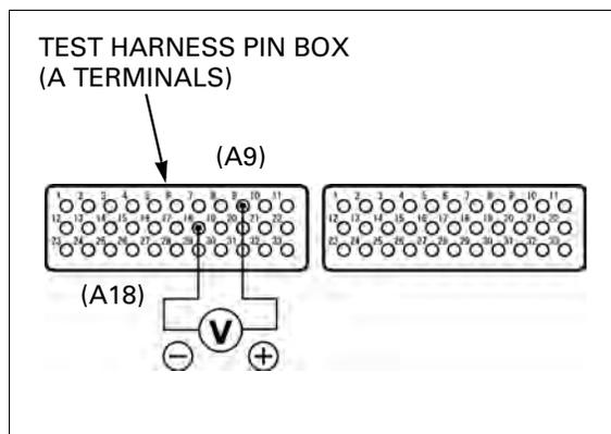
**4. TP Sensor Output Line Inspection**
