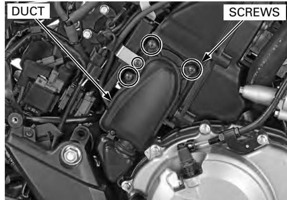
Install the right front resonator and tighten the screw securely.
