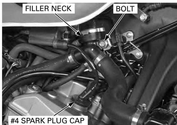
Loosen the hose band screw and disconnect the water hose from the filler neck.
