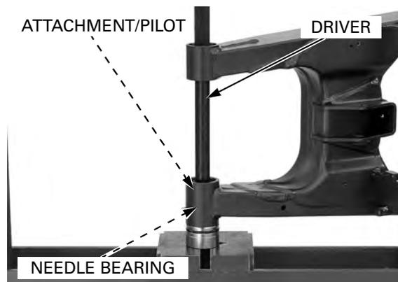
Press the left pivot needle bearing in until the depth from the swingarm outer surface is 8 – 9 mm (0.31 – 0.35 in) using the special tools and a hydraulic press.
