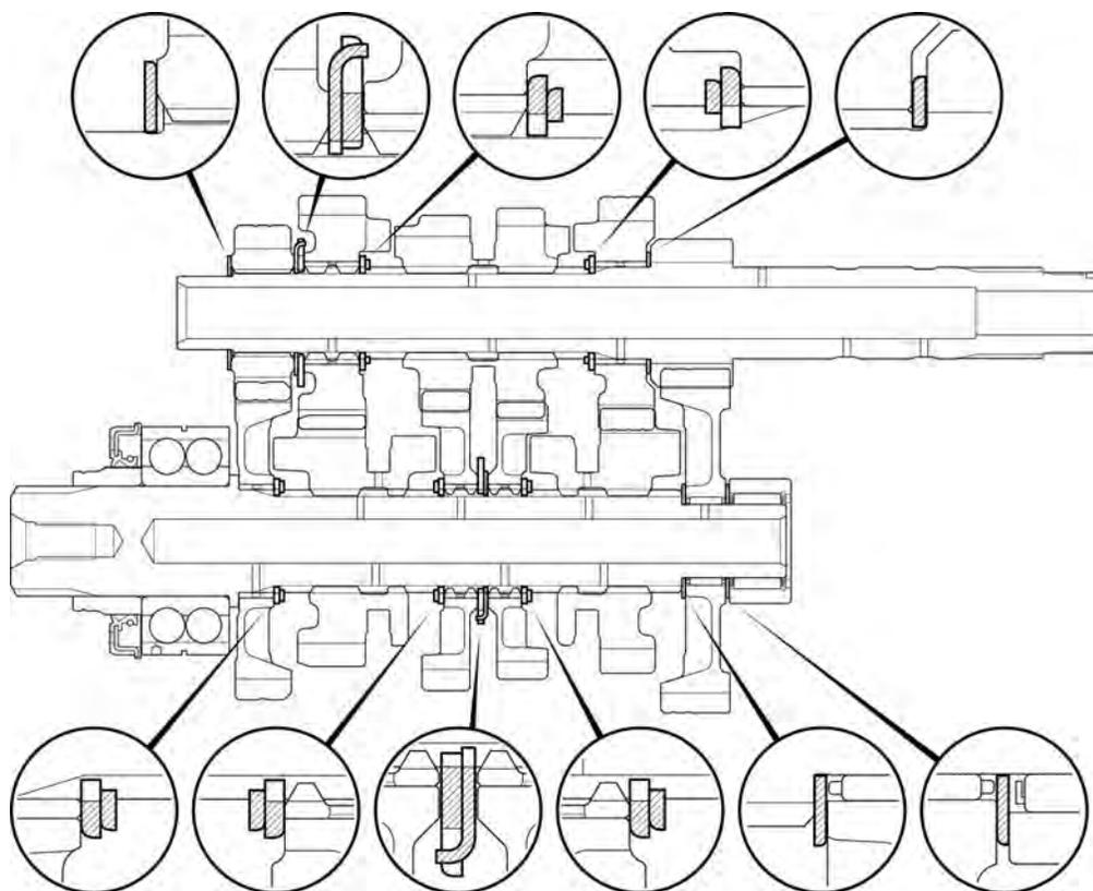
Assemble the transmission gear and shafts.
