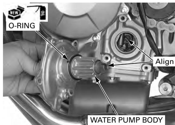
Align the mounting bolt holes in the water pump and crankcase and make sure the water pump is securely installed.
