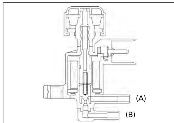
Check the resistance between the terminals of the IDC solenoid valve.
