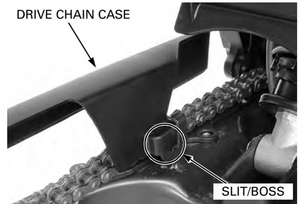
Tighten the drive chain case bolts to the specified torque.
