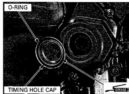
Tighten the timing hole cap to the specified torque.
