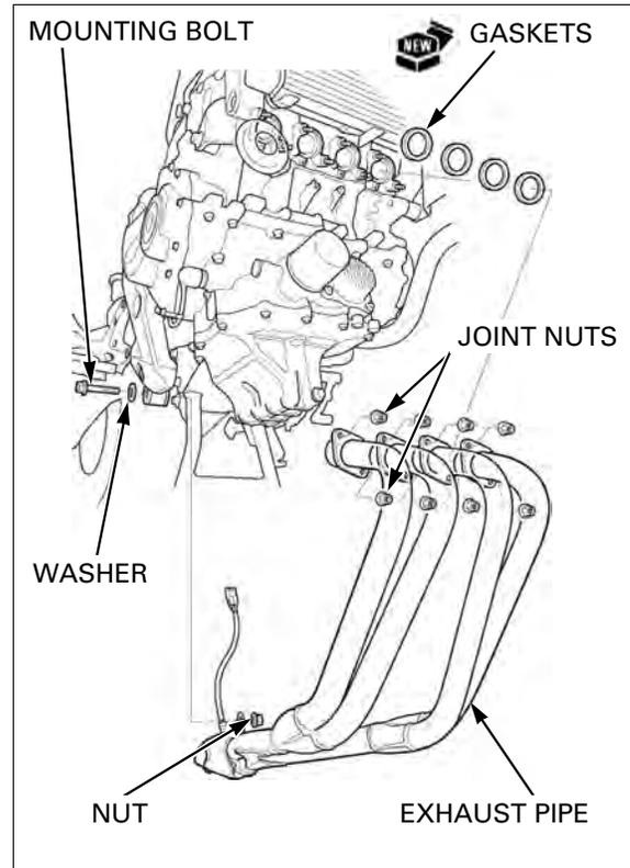
First tighten the exhaust pipe joint nuts to the specified torque.
