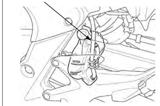
Install mounting bolt with the collar, then tighten the bolt securely.
