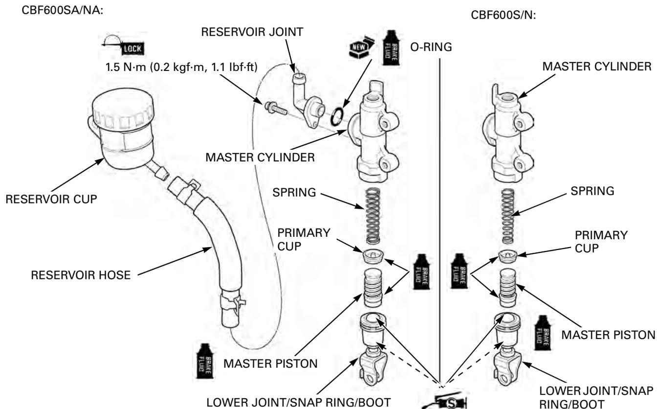
Apply silicone grease to the piston contacting surface of the push rod.
