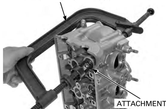
*Support the cylinder head above the work bench surface to prevent possible valve damage.*
