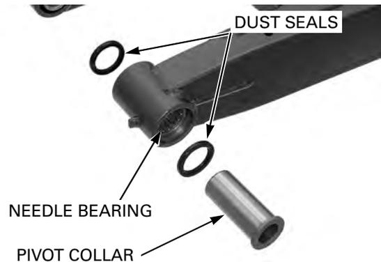
Remove the pivot side collars and dust seals from the swingarm right pivot.
