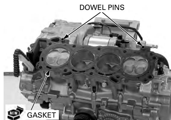
Install the cylinder head onto the cylinder block while aligning the cam chain tensioner A and B as shown.
