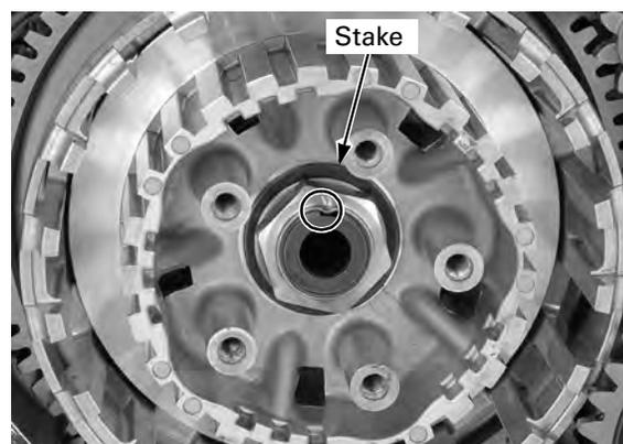
Install the spring seat and judder spring onto the clutch center as shown.
