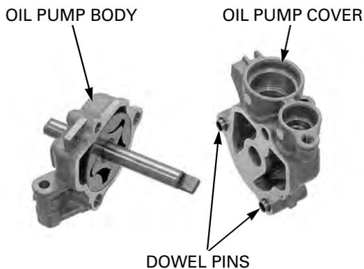
Remove the thrust washer, drive pin, oil pump shaft, outer rotor and inner rotor from the oil pump body.
