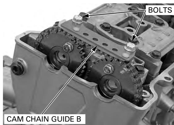
*Suspend the cam chain with a piece of wire to prevent the chain from falling into the crankcase.*
