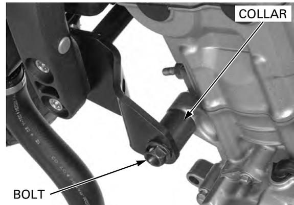
Tighten the right and left front engine hanger bracket nuts to the specified torque.
