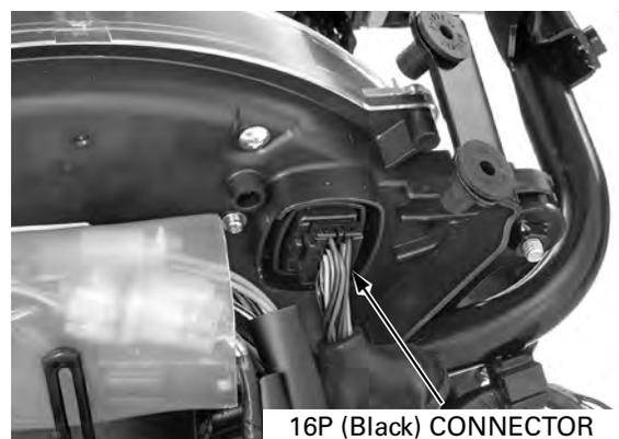
Connect the peak voltage adaptor to the tachometer Yellow/green (+) terminal and Green/black (-).
