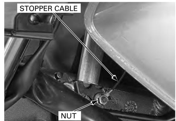
Remove the nut and pivot bolt, then remove the fuel tank.
