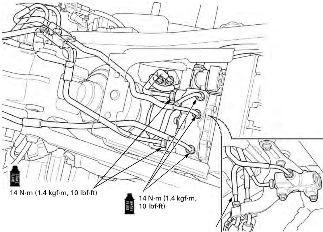
Installation is in the reverse order of removal by loosely tightening all the fasteners.
