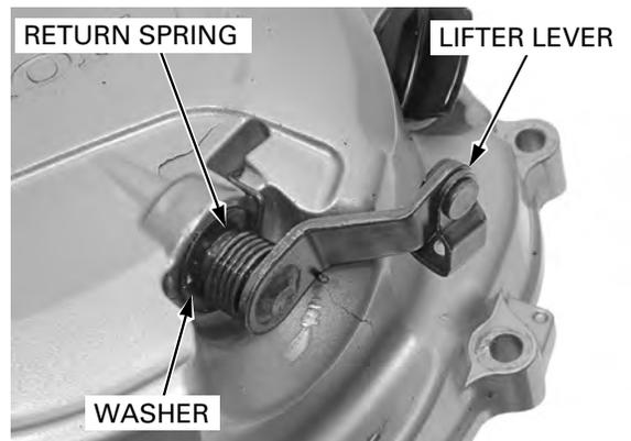
Check the lifter lever oil seal and needle bearings for wear or damage.
