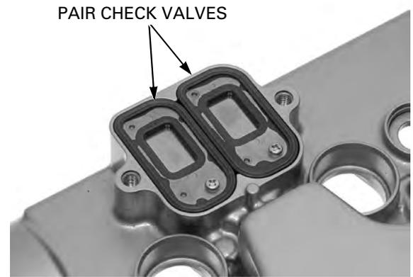
Install the PAIR check valve cover and tighten the bolts to the specified torque.
