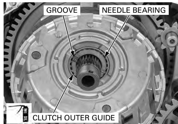
Install the thrust washer.
