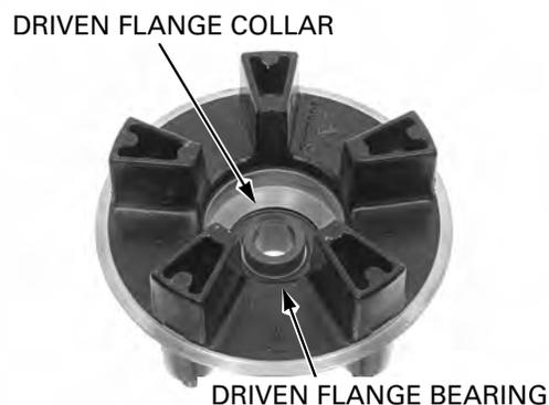
Drive out the driven flange bearing using the special tool.
