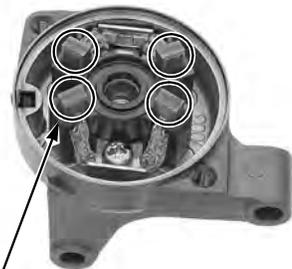
Install the armature to the rear cover.
