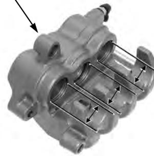
Check the caliper pistons for scratches, scoring or other damage.
