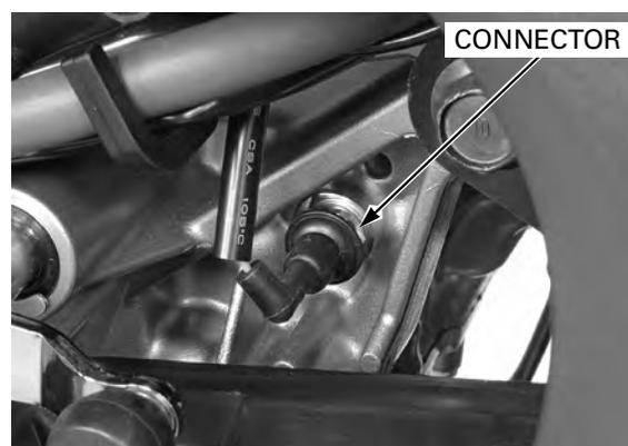
Remove the neutral switch and sealing washer.
