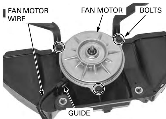
Install the cooling fan onto the fan motor shaft by aligning the flat surfaces.
