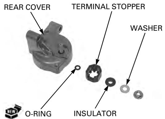
Install and tighten the terminal nut securely.
