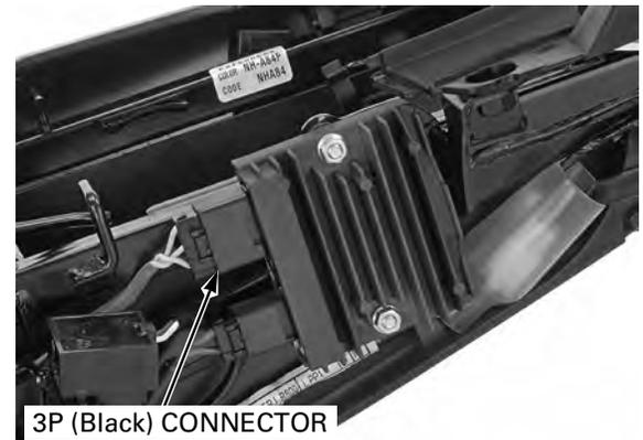
Release the alternator wire from the clamps.
