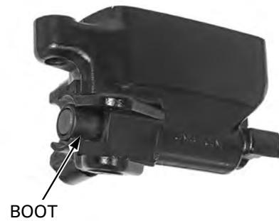
Remove the snap ring from the master cylinder body using the special tool.
