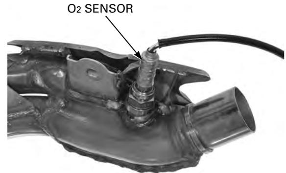
Remove the O<sub>2</sub> sensor using the special tool.
