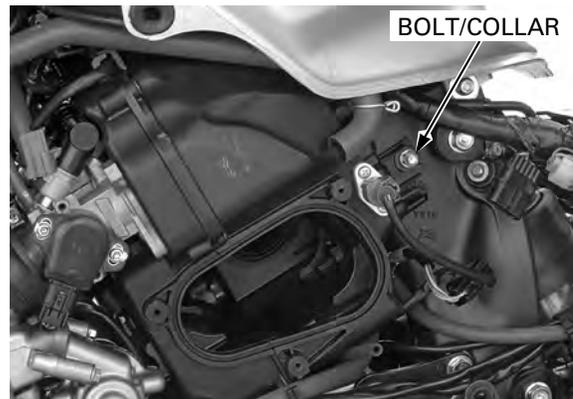
Connect the PAIR control solenoid valve 2P (Black) connector.
