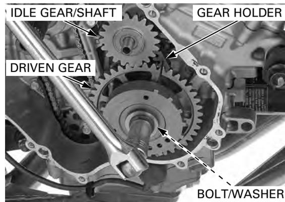
Remove the starter clutch outer assembly.
