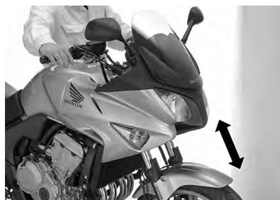
Check for worn steering stem bearings by grabbing the front fork leg and attempting to move the front fork side to side.
