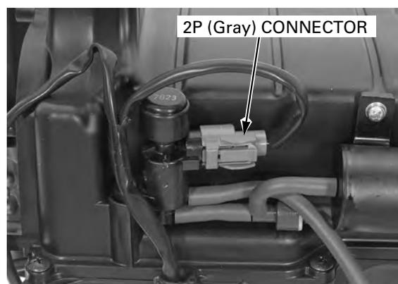
Disconnect the vacuum hoses and remove the screw and IDC solenoid valve.
