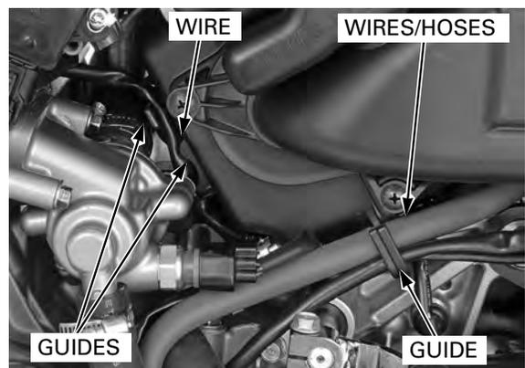
Remove the screws and left air cleaner duct from the air cleaner housing.
