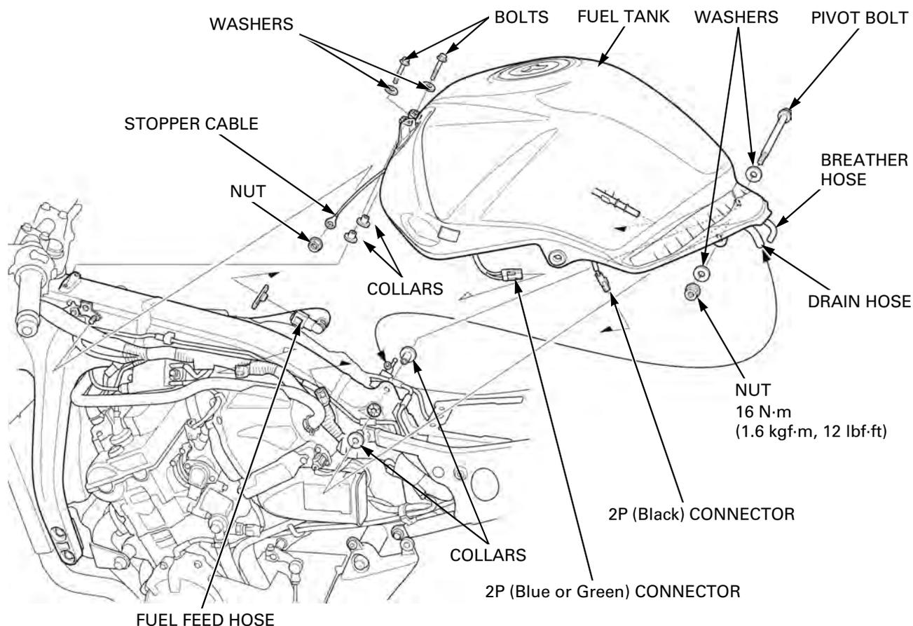
Install the fuel tank onto the frame, then install the collars, washers pivot bolt and nut.
