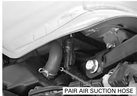
Release the wires and hoses from the guides of air cleaner housing.
