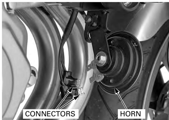
Remove the bolt, nut and horn.
