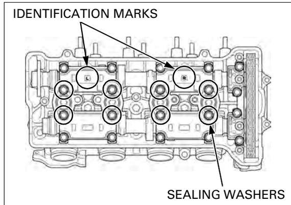
Gradually tighten the camshaft holder bolts until the camshaft holders lightly contact the cylinder head surface.
