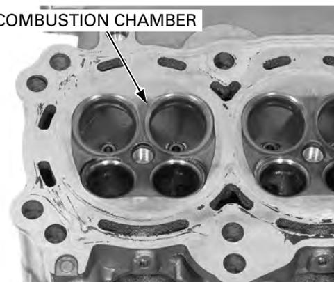
Check the cylinder head for warpage with a straight edge and feeler gauge.
