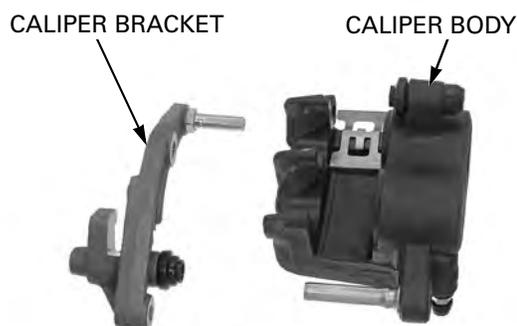
Remove the pad retainer and caliper pin boot from the caliper bracket.
