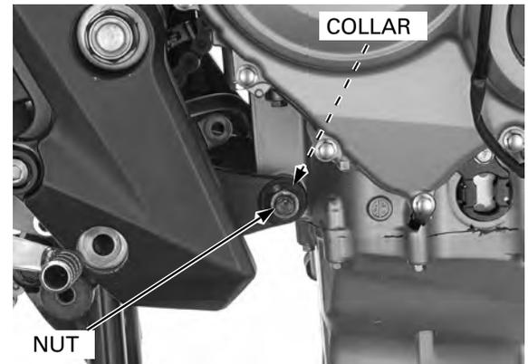
Remove the rear lower engine mounting bolt as shown.
