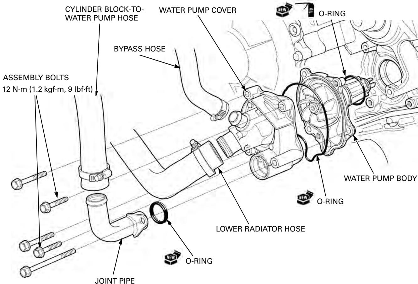
Apply engine oil to a new O-ring and install it onto the stepped portion of the water pump body.
