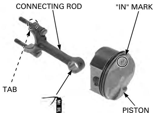
Install the piston pin and secure it using new piston pin clips.
