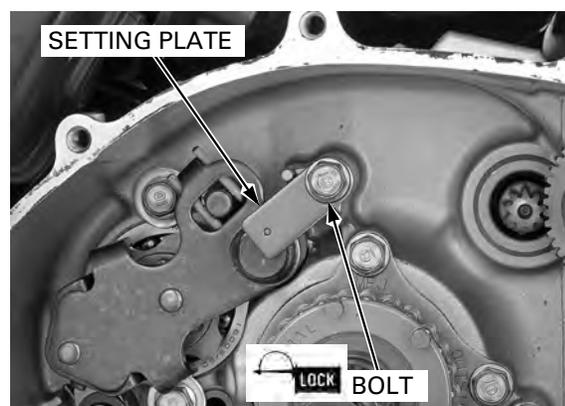
Install the gearshift arm to the gearshift spindle, aligning the arm slit with the punch mark on the gearshift spindle.
