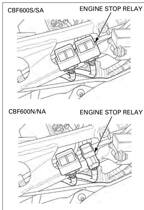
Connect the ohmmeter to the engine stop relay connector terminals.
