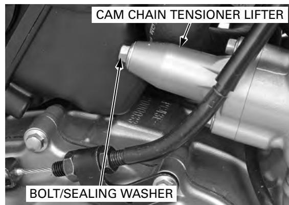
Turn the cam chain tensioner lifter shaft fully in (clockwise) and secure it using the special tool to prevent damaging the cam chain.
