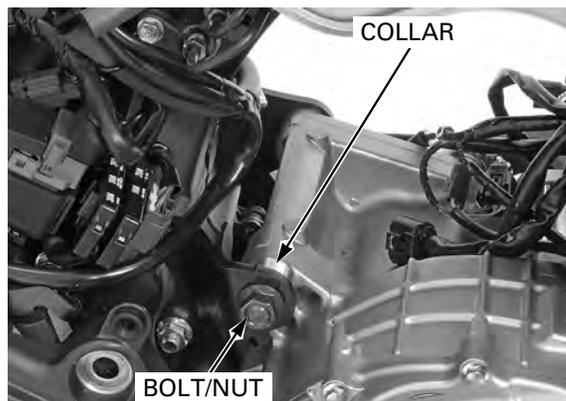
*Install the collar onto the right side engine mount.*
