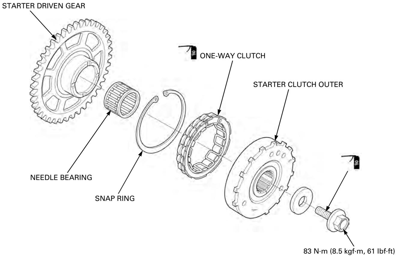
Apply engine oil to the one-way clutch.
