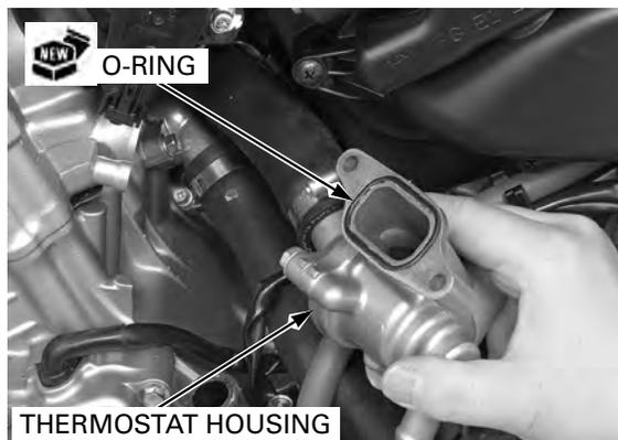
Install the thermostat housing to the cylinder head and tighten the bolts securely.
