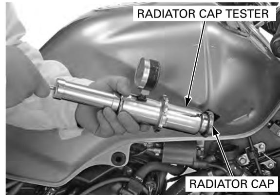
Pressure the radiator, engine and hoses, and check for leaks.
