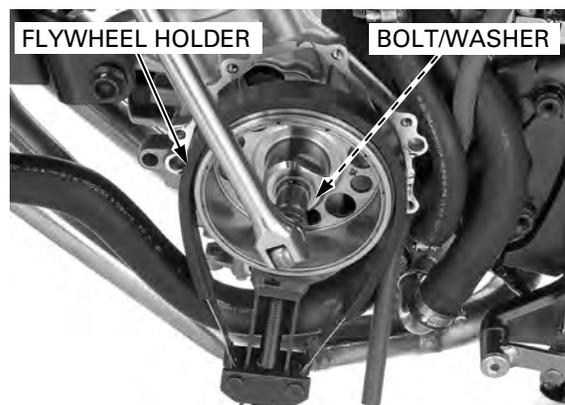
Remove the flywheel using the special tool.
