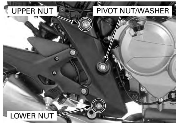
Install and tighten the swingarm pivot nut to the specified torque.
