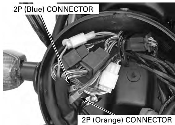
Remove the mounting nut and turn signal unit.
