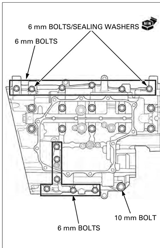
Place the engine with the lower side down.
