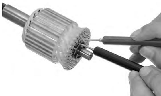
Check for continuity between each individual commutator bar and armature shaft. There should be no continuity.
