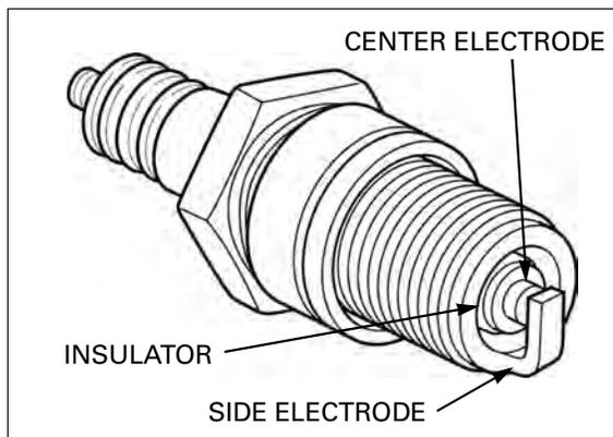
Check the gap between the center and side electrodes with a wire-type feeler gauge.
