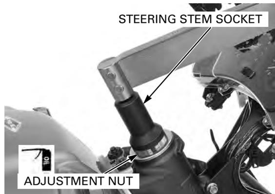
Move the steering stem right and left, lock-to-lock, five times to seat the bearings.
