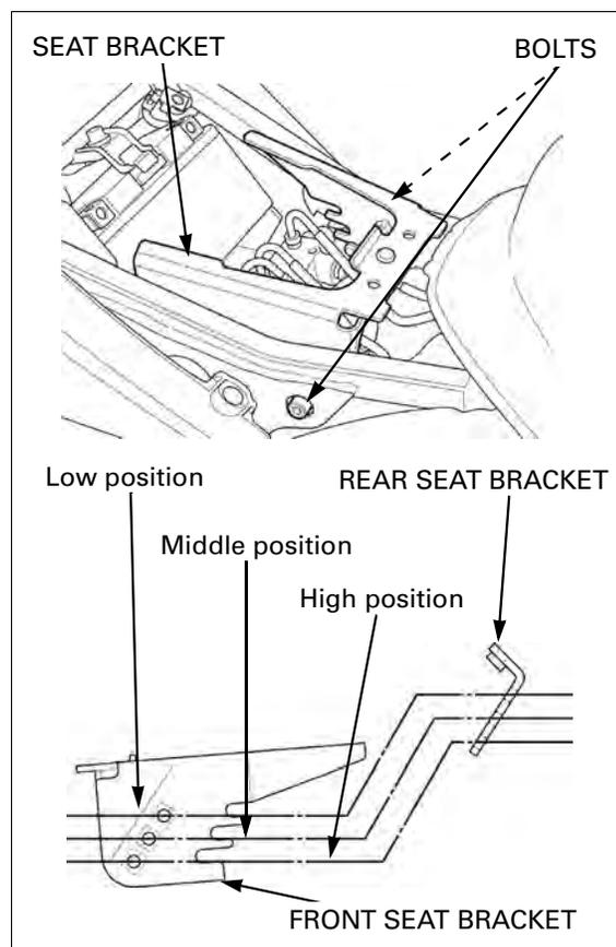
Remove the bolts and rear seat bracket.
