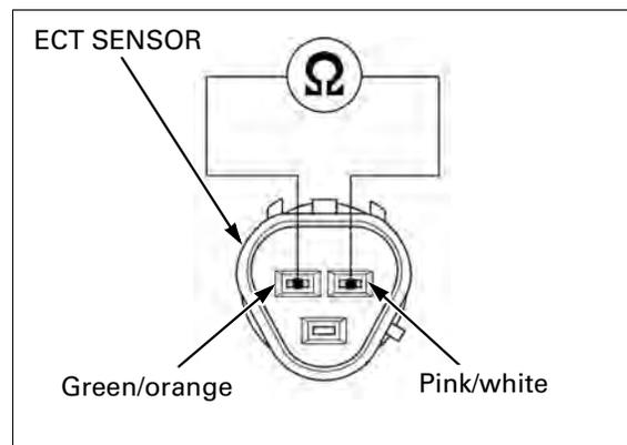
**4. ECT Sensor Short Circuit Inspection**
