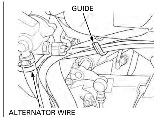
Secure the alternator wire with the clamps.
