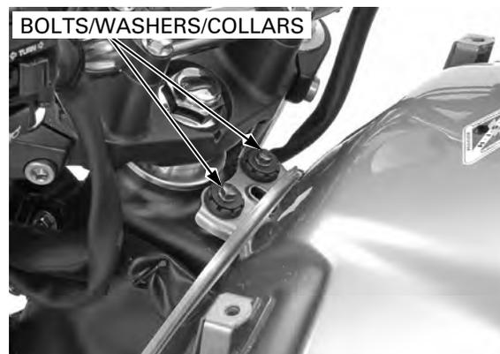
Lift the fuel tank and support it using the equipped tools (eye wrench and handle) as shown.
