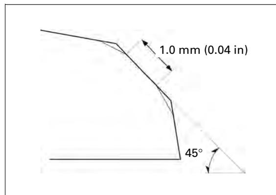
After cutting the seat, apply lapping compound to the valve face, and lap the valve using light pressure.
