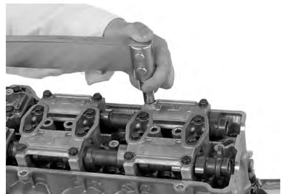
Install the cam chain guide B, and tighten the bolts.
