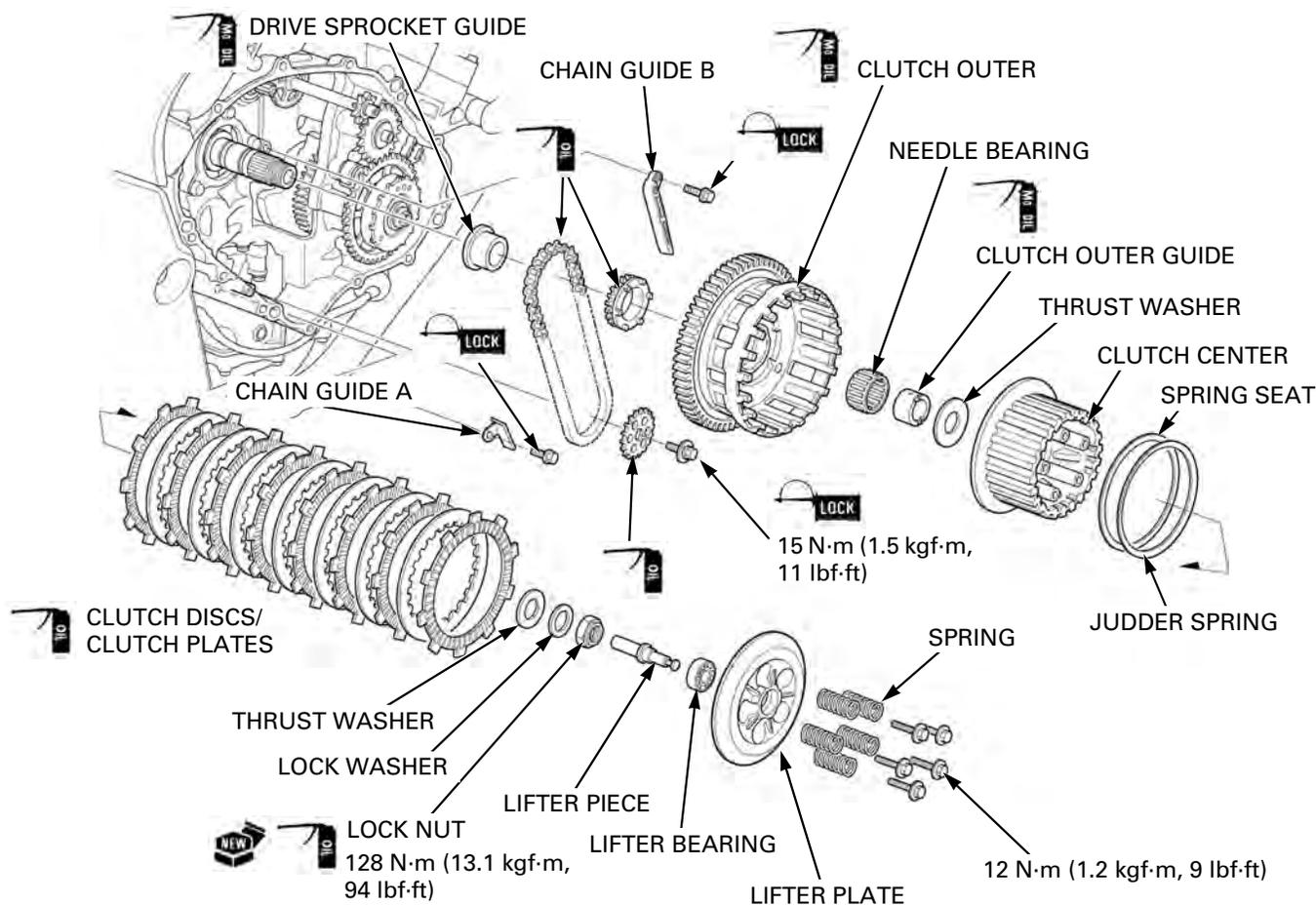
Apply molybdenum oil solution to the oil pump drive sprocket guide sliding surface and install it to the mainshaft.
