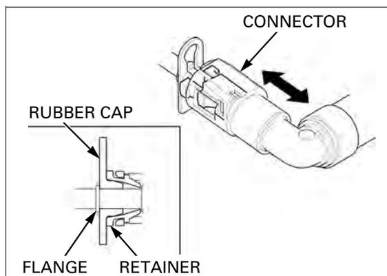
5. Connect the fuel pump 2P (Black) connector and clamp the wire.
