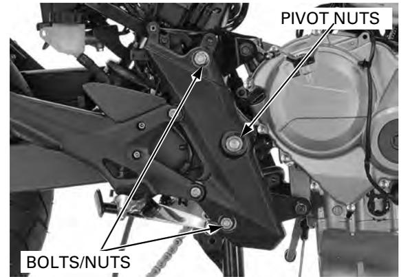
Remove the rear lower engine mounting nut and collar.
