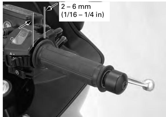
Throttle grip freeplay can be adjusted at either end of the throttle cable.
