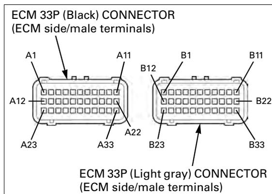
The ECM test harness terminals are same layout as for the ECM connector terminals as shown.
