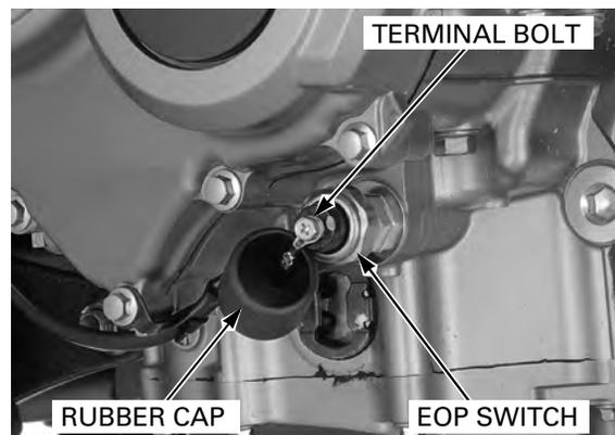
Install the oil pressure gauge attachment to the switch base.
