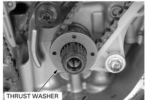
Install the starter clutch outer assembly into the crankshaft while aligning the tab of the crankshaft with the wide groove of the starter clutch assembly.
