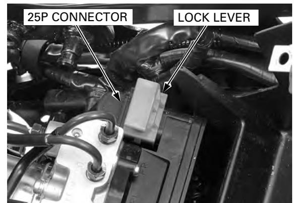
*When loosening the joint nuts, cover the end of the brake pipes to prevent contamination.*
