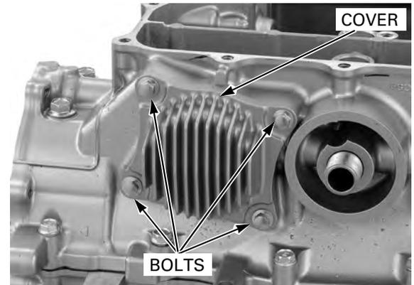
Remove the bolts and sealing washers.
