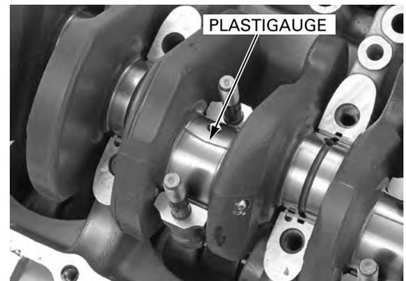
Carefully install the connecting rod bearing caps by aligning the I.D. code.
