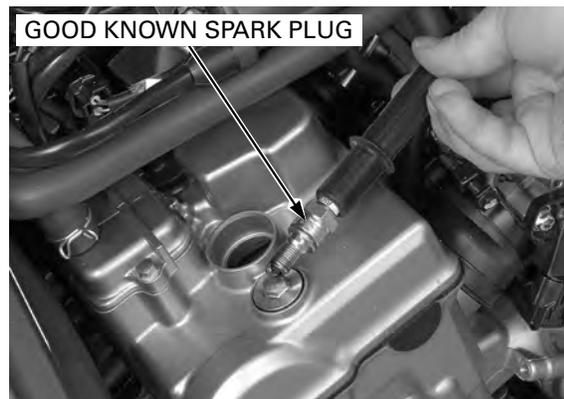
With the ignition coil primary wire connected, connect the peak voltage adaptor or peak voltage tester to the ignition coil primary wire terminals.
