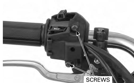
Pull the clutch lever and install the clutch switch with its hook to the groove on the clutch lever bracket. Connect the clutch switch wire connectors to the switch.
