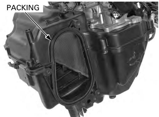
Remove the right air cleaner duct packing.
