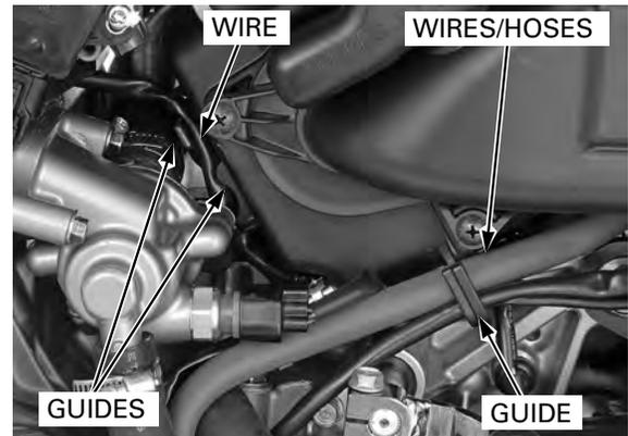
Connect the PAIR air suction hose to the air cleaner housing.
