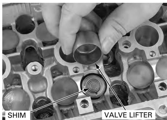
Clean the valve shim contact area in the valve lifter with compressed air.
