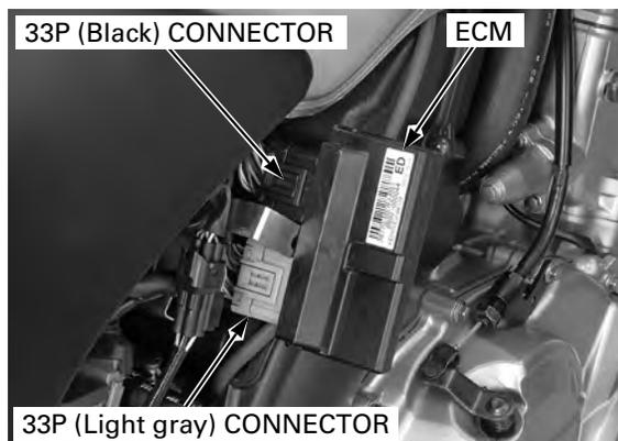
Connect the ECM test harness between the main wire harness and the ECM.
