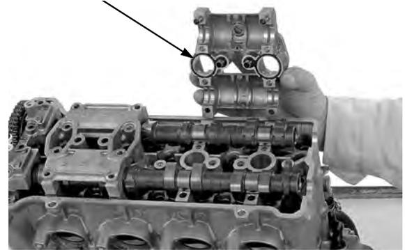
Apply engine oil to the threads and seating surfaces of the camshaft holder bolts.
