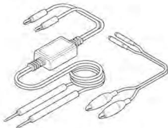
with commercially available digital multimeter (impedance 10 M $\Omega$ /DCV minimum) or Imrie diagnostic tester (model 625)
