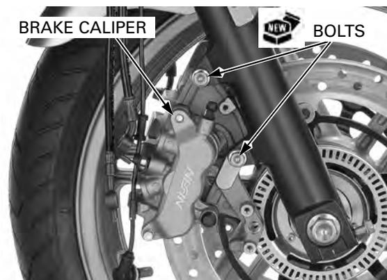
Install the front wheel speed sensor (page 16-24).
