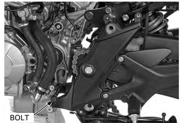
Remove the rear upper engine mounting bolt/nut and collar.
