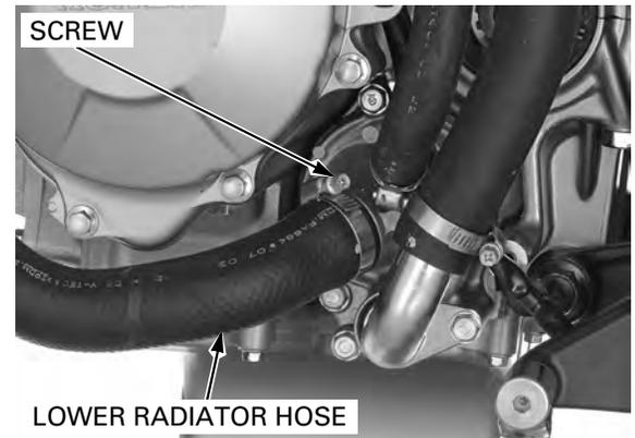
Remove the radiator lower mounting bolt and washer.
