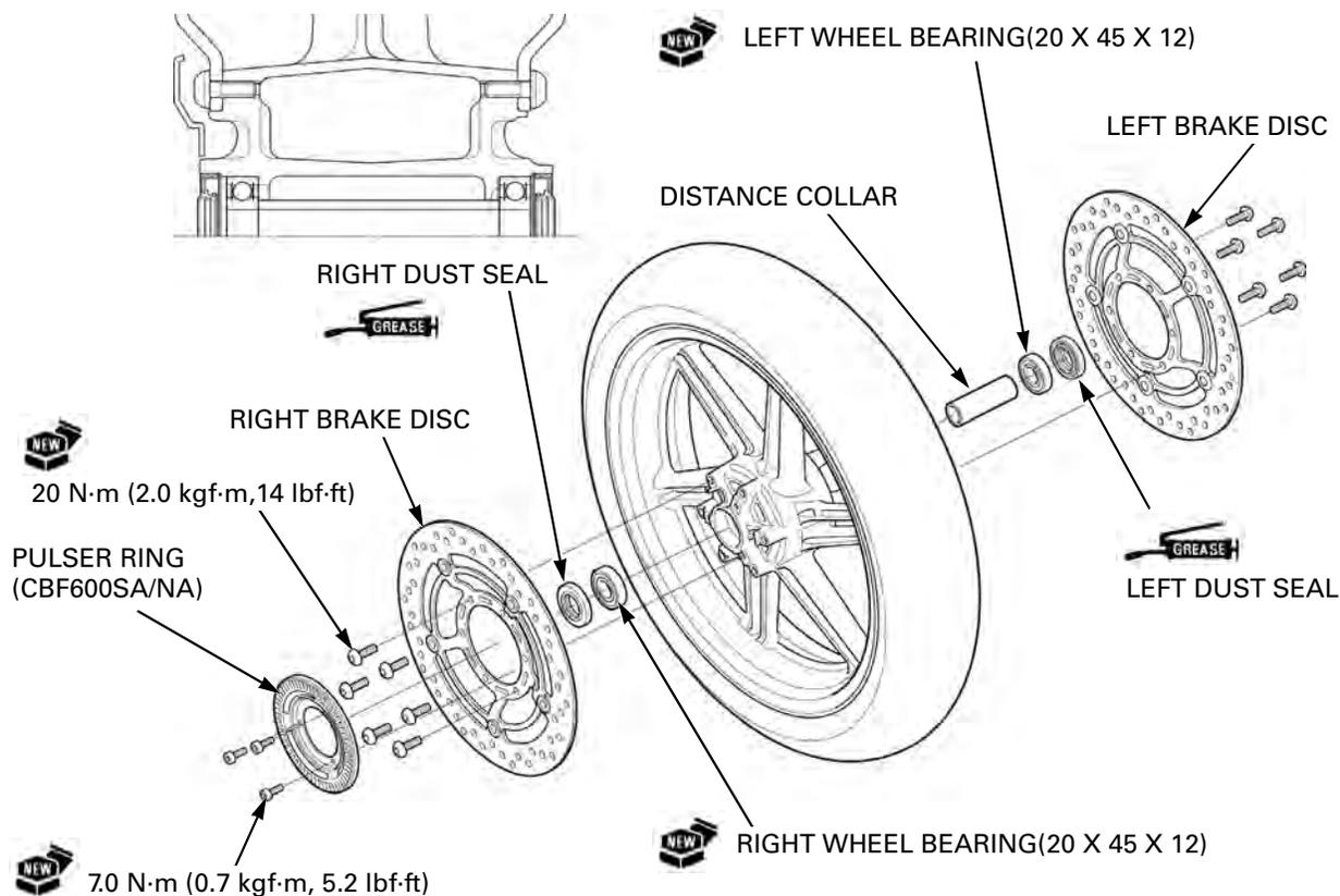
Never install the old bearings. Once the bearings has been removed, the bearing must be replaced with new ones.
