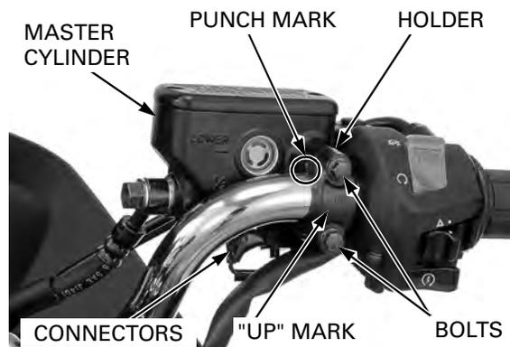
Install the clutch lever bracket by aligning the punch marks on the handlebar and bracket.
