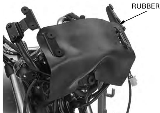
Disconnect the ignition switch 2P (Brown) connector and immobilizer 4P connector.
