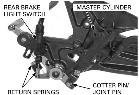
Remove the snap ring, washer and brake pedal.
