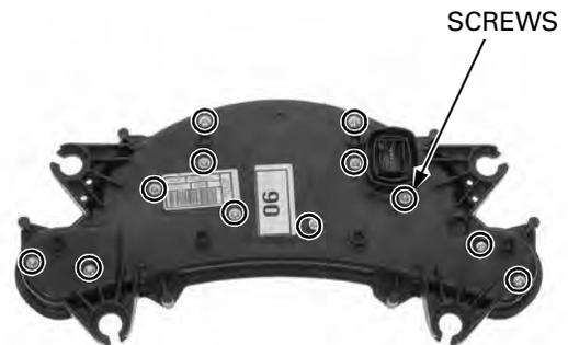
Install the clear cover, then tighten the screws securely.
