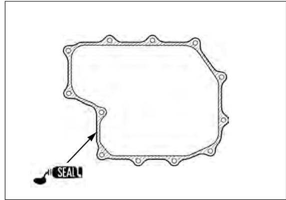
Install the oil pan onto the lower crankcase.
