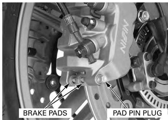
Remove the pad pin and brake pads.
