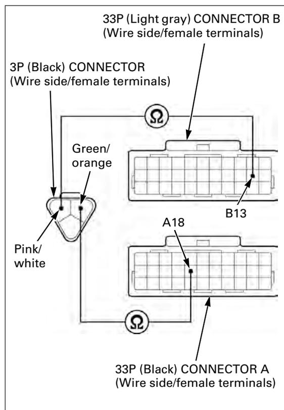
**DTC 8-1 (TP SENSOR LOW VOLTAGE)**
