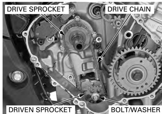
Remove the oil pump drive sprocket guide.
