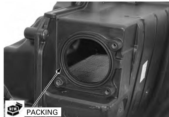
Install a new left air cleaner duct packing into the groove on the housing.
