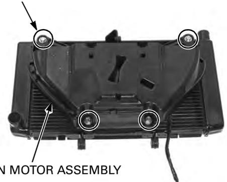
Remove the nut and cooling fan.
