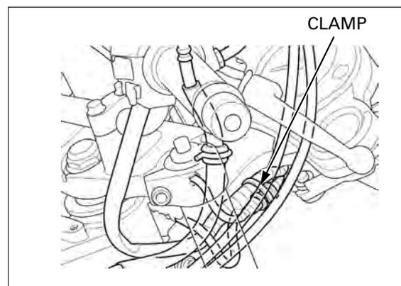
Release the wire clamp and remove the main wire harness and left handlebar switch wire.
