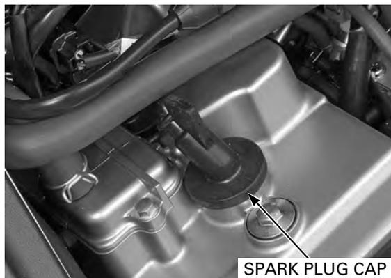
Remove the spark plugs using a equipped spark plug wrench or an equivalent tool.
