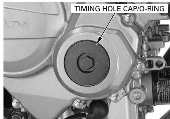
Turn the crankshaft clockwise, align the "T" mark on the CKP sensor rotor with the index mark on the right crankcase cover.
