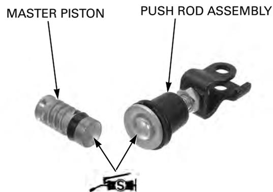
Coat all parts with clean brake fluid before assembly.
