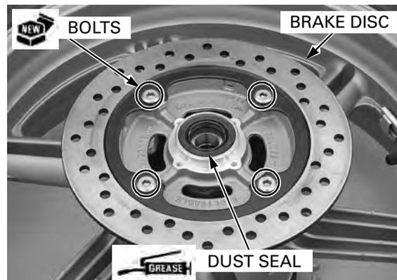
*CBF600SA/NA only* Install the pulser ring. Install and tighten the new mounting bolts to the specified torque.
