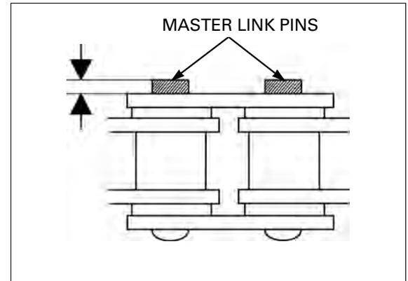
Make sure that the pins are staked properly by measuring the diameter of the staked area using a slide caliper.
