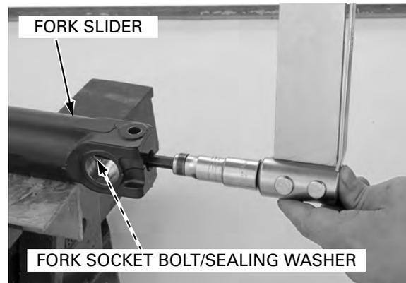
Install the axle holder bolt to the fork slider, but do not tighten yet.
