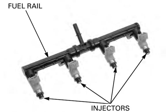
Remove the seal ring and O-ring from each injector.
