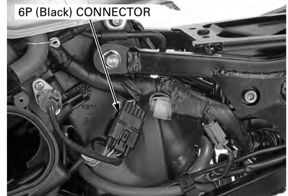
Disconnect the #2/#3 ignition coil connectors.
