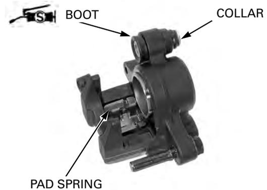
Install the pad retainer and caliper main slide pin boot into the caliper bracket.
