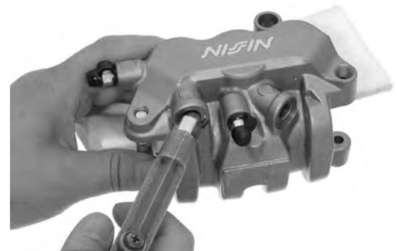
*Be careful not to damage the piston sliding surface.*
