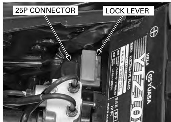
**3. Indicator Signal Line Short Circuit Inspection**
