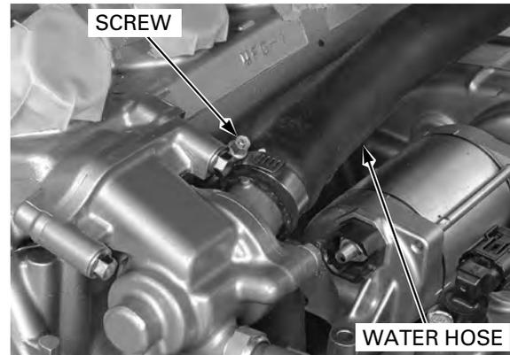
Loosen the hose band screw and disconnect the air bleed hose from the hose joint on the cylinder head.
