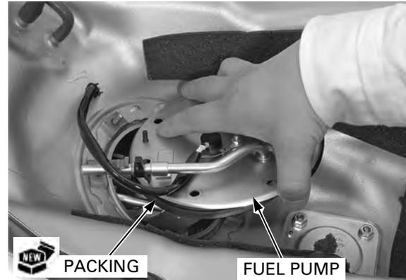
Install the fuel pump mounting nuts. Tighten the nuts in the specified sequence as shown.
