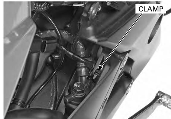
Connect the rear brake light switch 2P (Black) connector.
