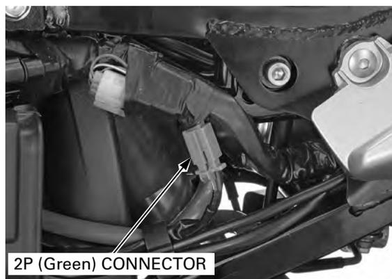
Check for continuity between the wire terminals of the sidestand switch 2P (Green) connector. Continuity should exist only when the sidestand is UP.
