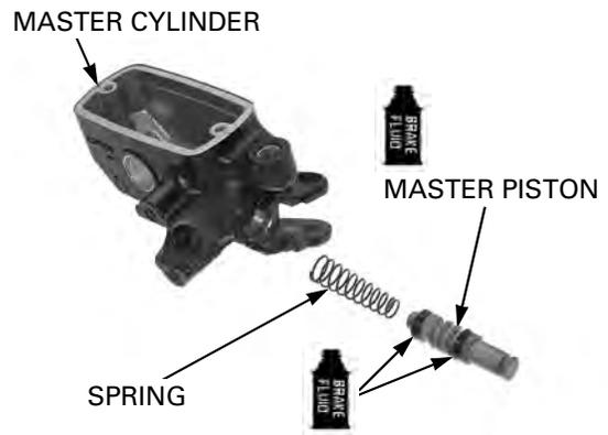
*Do not allow the piston cup lips to turn inside out.*
