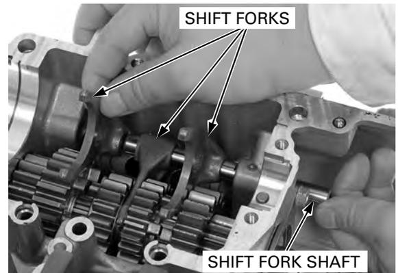
Remove the shift drum and shift drum bearing.
