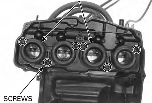
Remove the rubber seals from the lower air cleaner housing.
