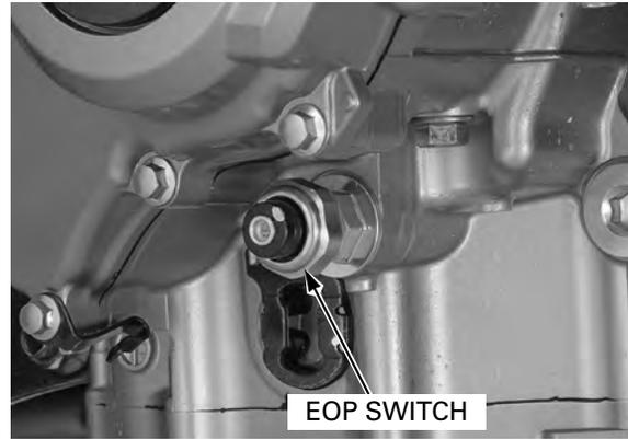
Connect the EOP switch wire and tighten the terminal bolt to the specified torque.
