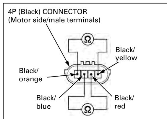
**DTC 33-2 (EEPROM)****1. Recheck DTC**
