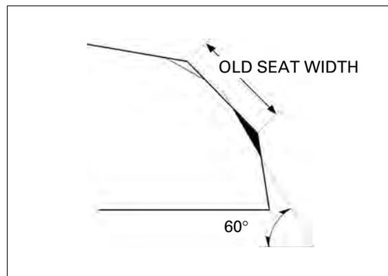
Using a 45-degree seat cutter, cut the seat to the proper width. Make sure that all pitting and irregularities are removed. Refinish if necessary.
