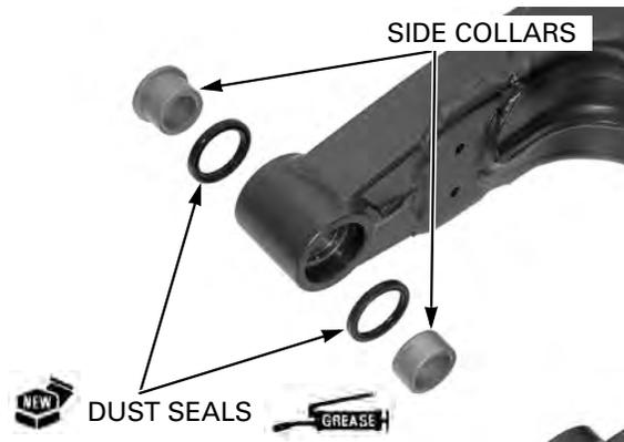
Apply grease to the dust seal lips, then install the dust seals and pivot collar into the left swingers pivot.
