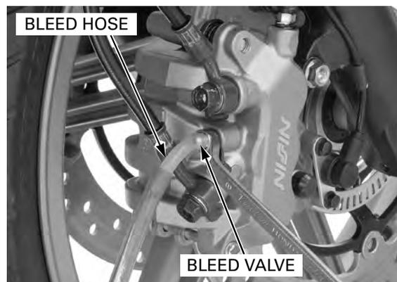
Connect a bleed hose to the rear caliper bleed valve. Loosen the bleed valve and pump the brake pedal until no more fluid flows out of the bleed valve.
