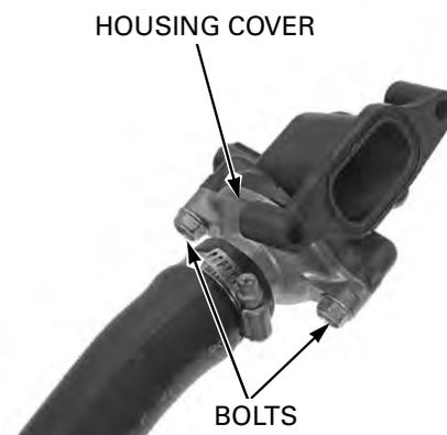
Remove the thermostat from the housing.
