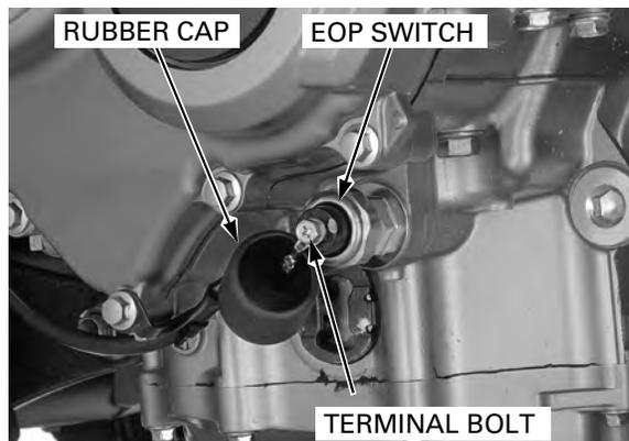
If the engine oil pressure and warning indicators do not function, check the following:
