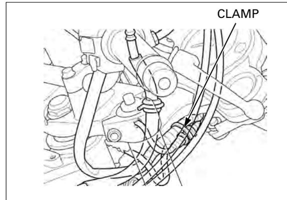
Connect the ignition switch 2P (Brown) connector and immobilizer 4P connector.
