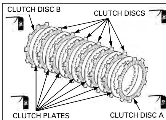
Install the tabs of outside clutch disc A into the shallow slots of the clutch outer.
