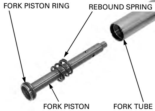
*Be careful not to scratch the fork tube or damage the dust seal.*
