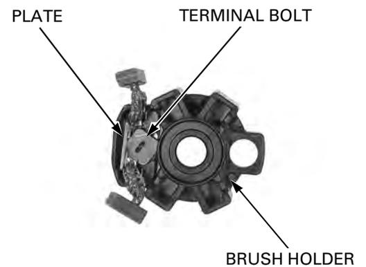
Disassemble the terminal bolt, positive brushes and brush holder.
