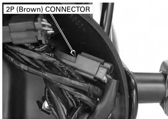
Check for continuity between the wire terminals of the ignition switch connector in each switch position.
