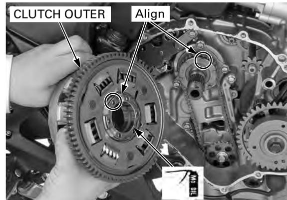
Apply molybdenum oil solution to the clutch outer guide sliding surface.
