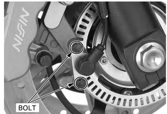
Remove the wheel speed sensor from the caliper bracket.
