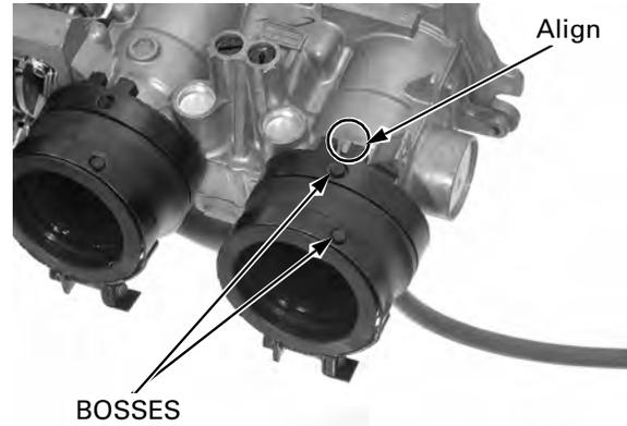
Confirm the direction of the insulator band screws as shown.
