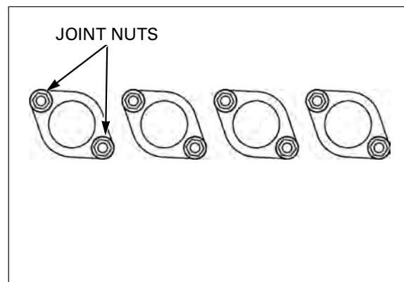
Tighten the exhaust pipe mounting nut to the specified torque.
