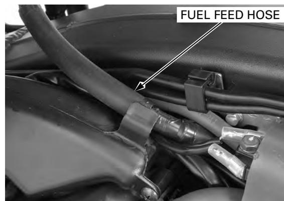
Remove a support tools, then lower the fuel tank.
