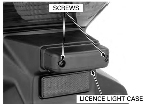
Remove the license light bulb and replace with a new one.
