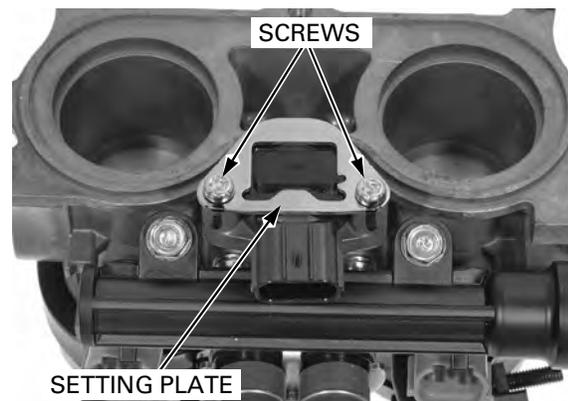
Remove the IACV motor and O-ring.
