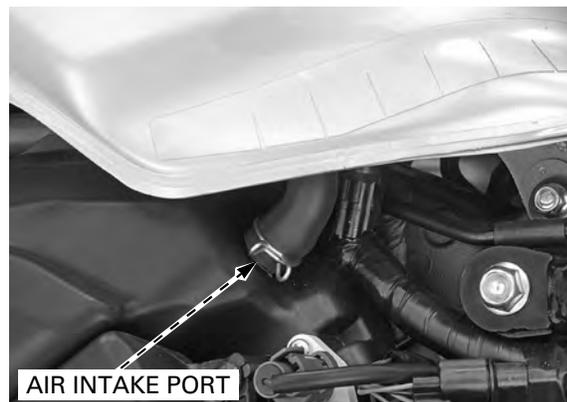
Start the engine and open the throttle slightly to be certain that the air sucked in through the air supply hose.
