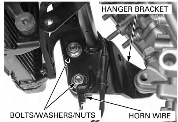
Install the left front engine hanger bracket bolts, washers and nuts.
