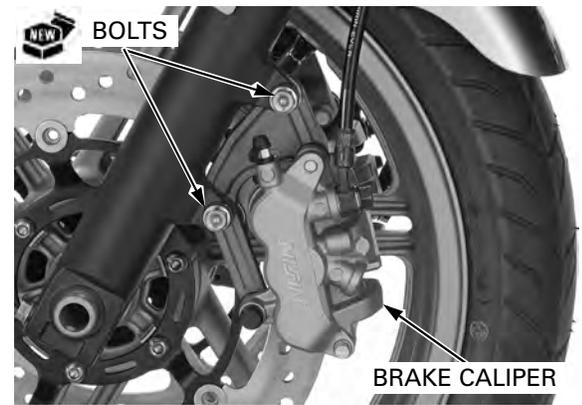
With the front brake applied, pump the fork up and down several times to seat the axle and check brake operation by applying the brake lever.
