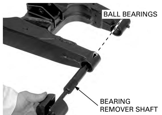
Press the left pivot needle bearing out using the special tools and a hydraulic press.
