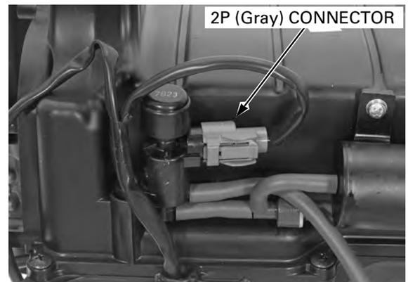
Install the IAT sensor with a new O-ring and tighten the screws securely.
