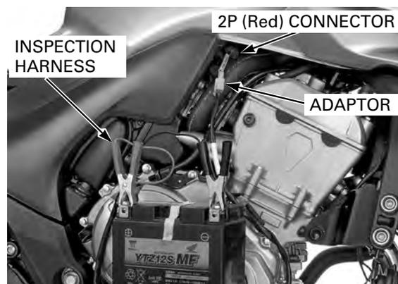
Turn the ignition switch to "ON" with the properly registered key.
