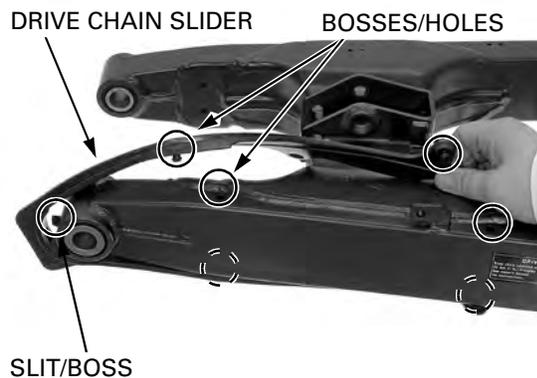
Install and tighten the drive chain slider bolts to the specified torque.
