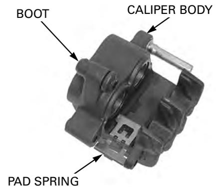
Install the brake pad retainer and caliper pin boot into the caliper bracket.
