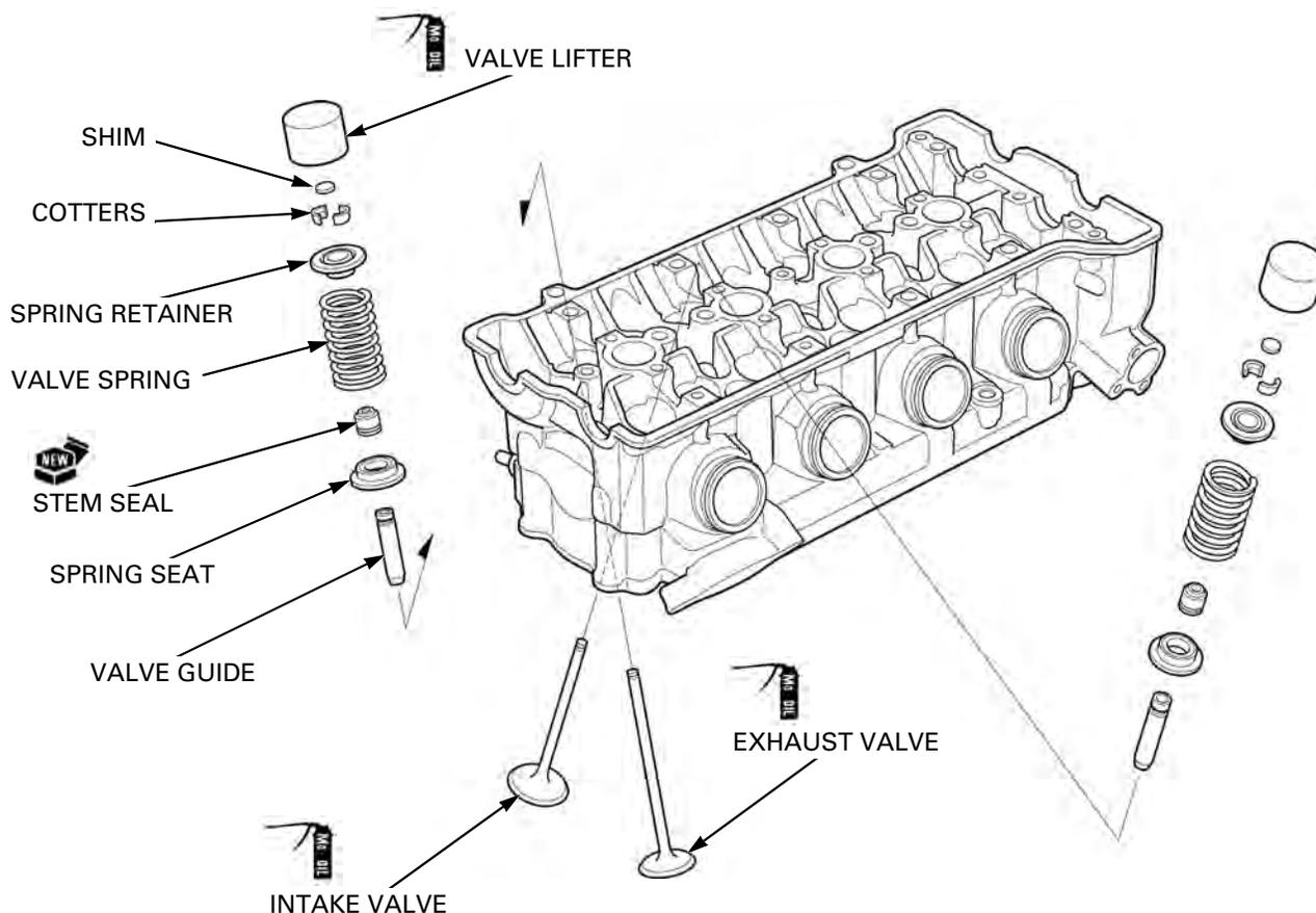
Blow through all oil passages in the cylinder head with compressed air.
