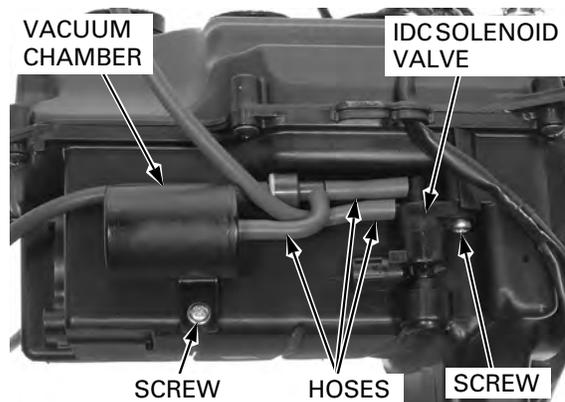
*Align the vacuum chamber boss with the hole on the air cleaner housing.*
