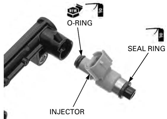
Install the injectors to the fuel rail.
