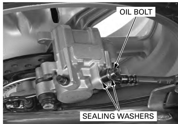
Pivot the caliper up and remove it.
