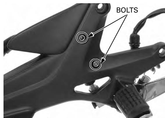
Install the right footpeg holder onto the frame, tighten the bolts to the specified torque.
