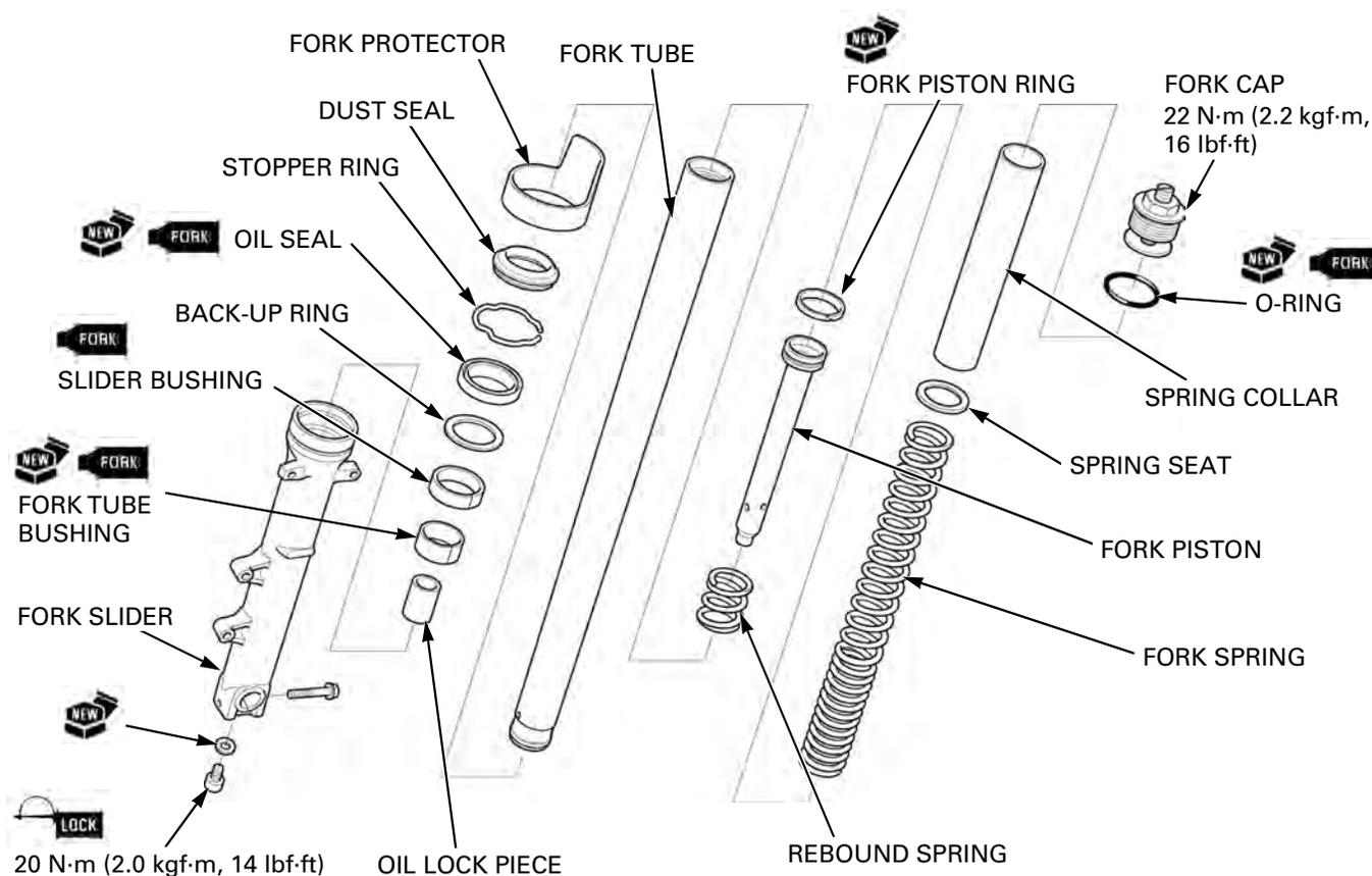
Before assembly, wash all parts with a high flash or non-flammable solvent and wipe them dry.
