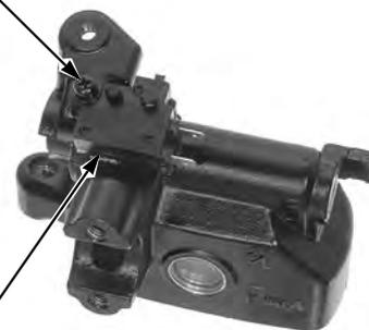
Apply silicone grease to the brake lever pivot bolt sliding surface.
