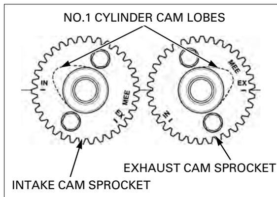
Clean and apply a locking agent to the cam sprocket bolt threads.
