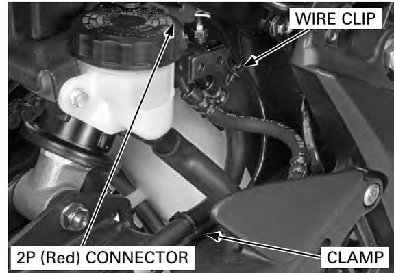
Release the sensor wire from the clamp.
