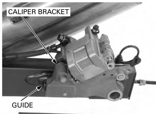
*Be careful not to damage the brake pads and speed sensor (CBF600SA/NA).*
