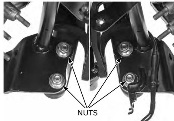
Tighten the lower engine mounting nut to the specified torque.
