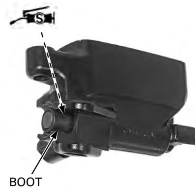
Apply silicone grease to the brake lever contacting surface of the master piston.
