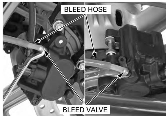
Pressurize the system with the brake lever until lever resistance is felt.
