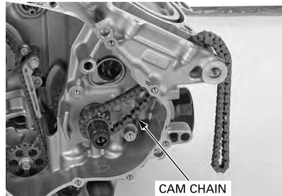
Install the cam chain guide A and bolt.
