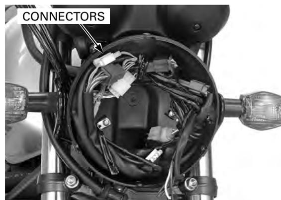
Remove the bolts, special nuts and headlight case.
