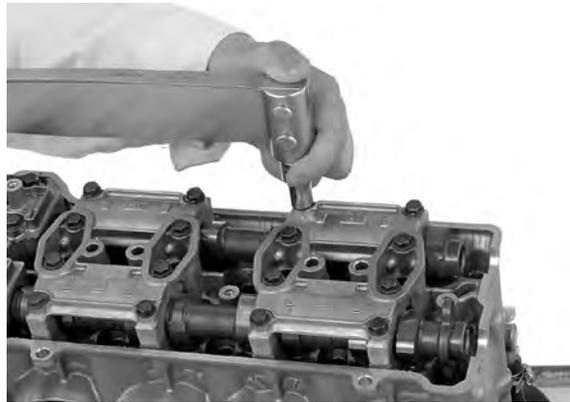
Remove the camshaft holders and measure the width of each plastigauge. The widest thickness determines the oil clearance.
