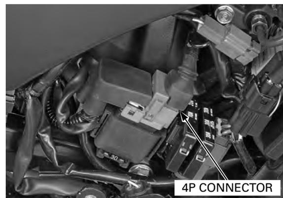
Remove the bolts and disconnect the starter relay cables.
