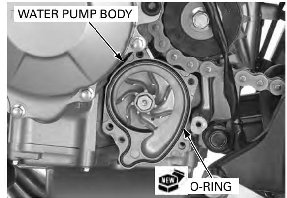
Install the water pump cover and mount bolts securely.
