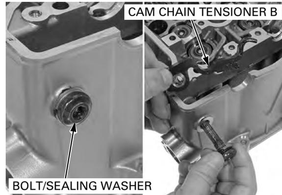
Remove the bleeding joint, sealing washer from the cylinder head.
