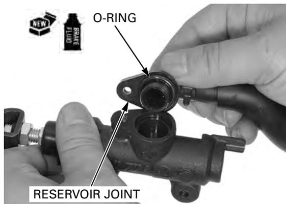
Apply a locking agent to the reservoir joint screw threads.
