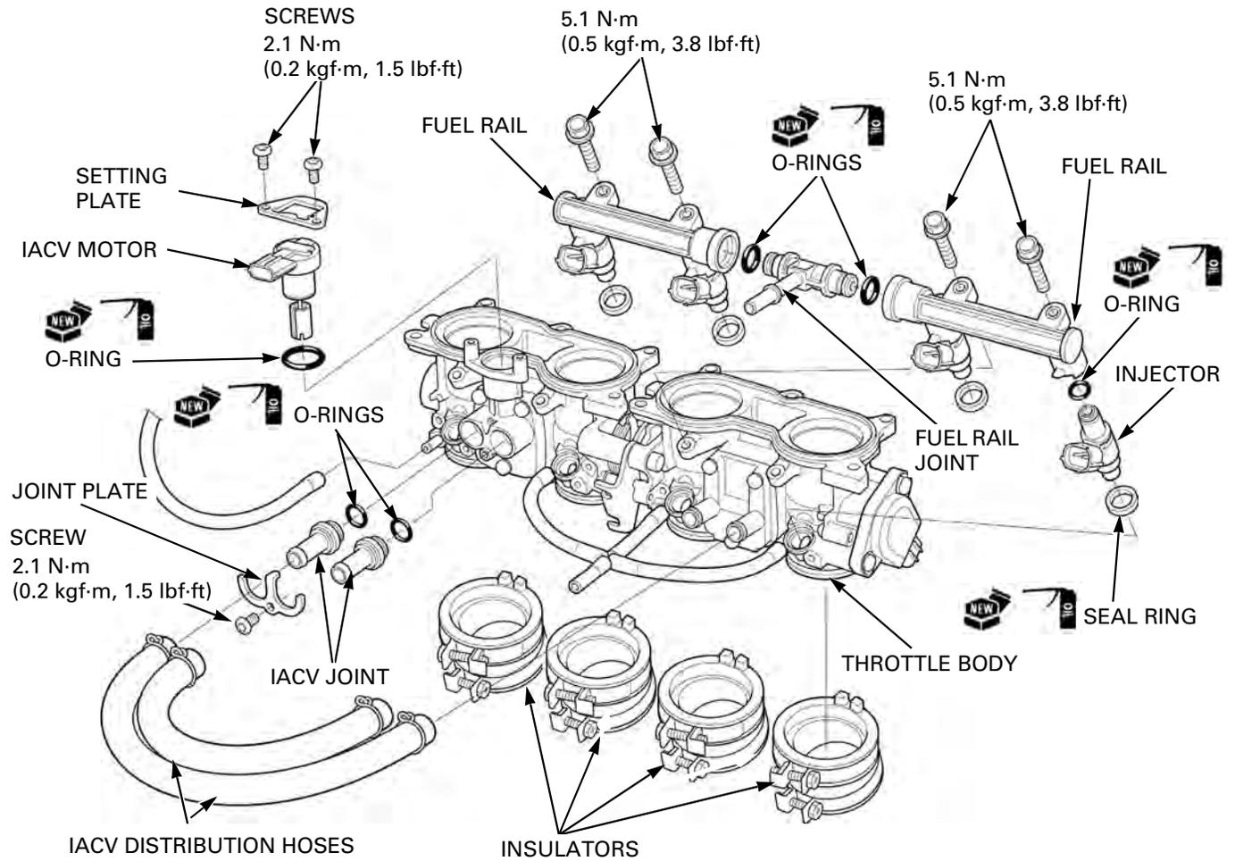
Apply oil to new O-rings of the fuel rail joint.
