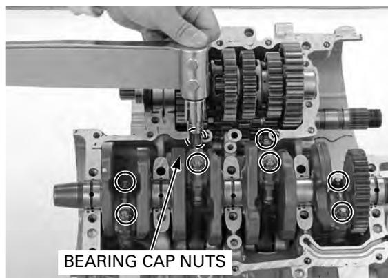
Remove the bearing caps and measure the compressed plastigauge at its widest point on the crankpin to determine the oil clearance.
