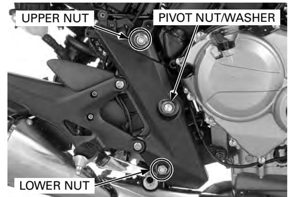
Slightly pull the pivot bracket outward.
