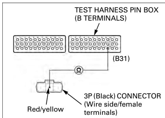
**5. TP Sensor Output Line Short Circuit Inspection**
