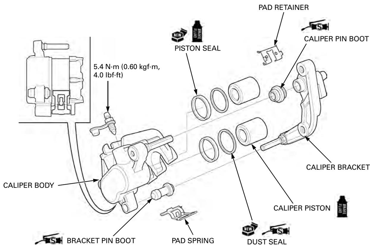
Coat new piston seals with clean brake fluid and install them into the seal grooves in the caliper.
