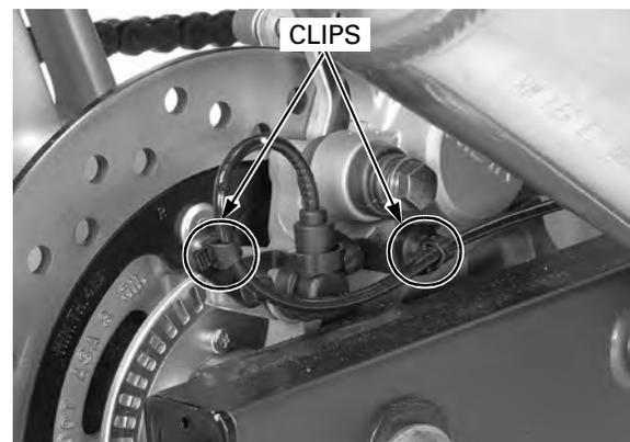
Remove the wheel speed sensor mounting bolts and guide.
