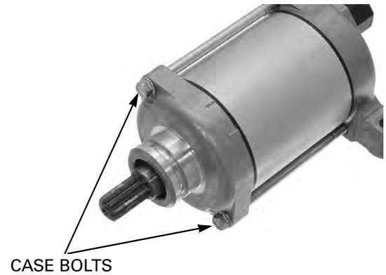
Remove the front cover and seal ring.
