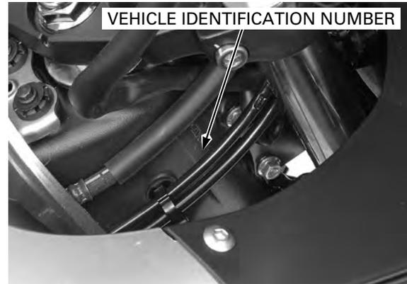
The registered number plate is located on left side of the frame tube.
