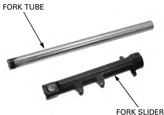
Place the fork tube in V-block and measure the runout. Actual runout is 1/2 the total indicator reading.
