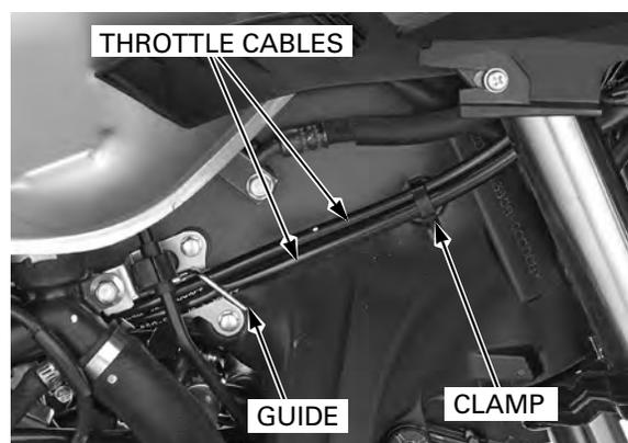
*CBF600S/SA only:* Secure the throttle cables with the clamp.
