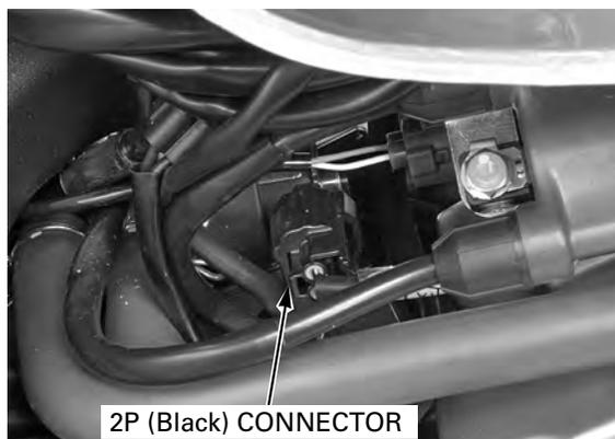
Pull the PAIR control solenoid valve out the stay.
