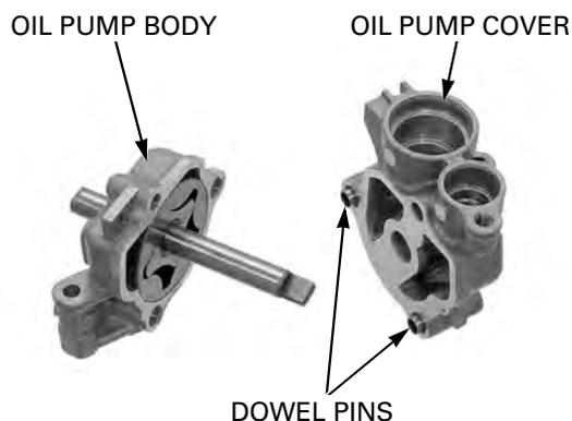
Install and tighten the oil pump assembly bolts to the specified torque.
