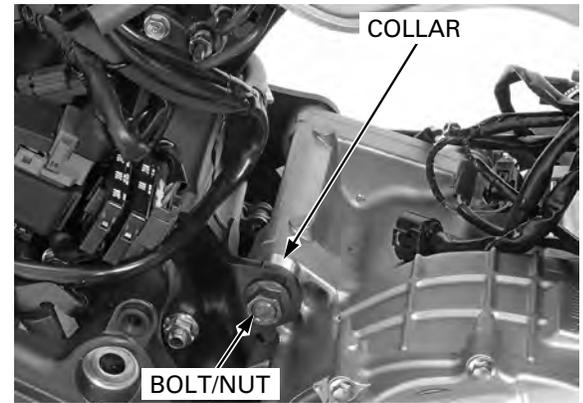
Tighten the right and left front engine mounting bolts to the specified torque.
