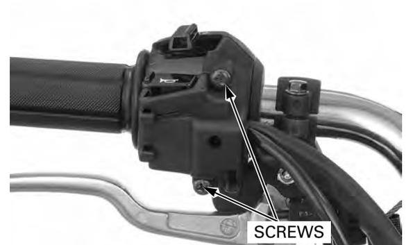
Remove the left handlebar switch housing.
