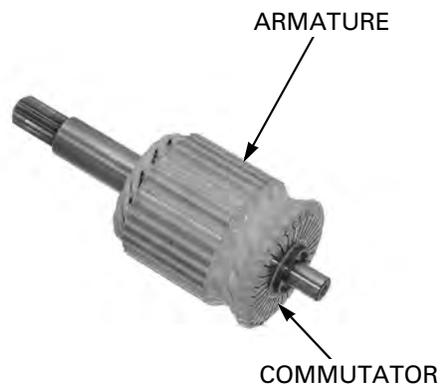
Check for continuity between pairs of commutator bars. There should be continuity.
