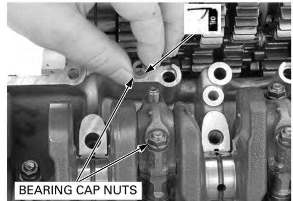
Tighten the nuts in two or three steps alternately, then tighten the nuts to the specified torque.
