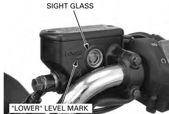
If the fluid level is near the "LOWER" level mark, remove the reservoir cap, set plate and diaphragm, and fill the reservoir with DOT 4 brake fluid from a sealed container to the casting ledge.
