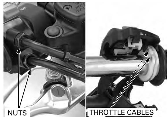
CBF600S/SA only: Release the throttle cables from the clamp.
