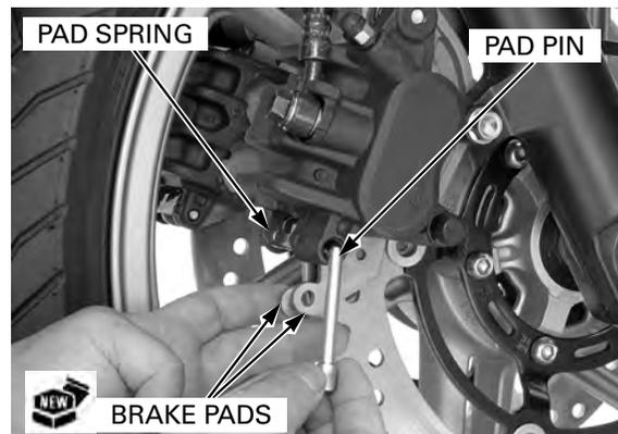
Tighten the pad pin to the specified torque.
